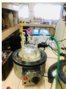
Fig.4.3:- Degassing of oil
