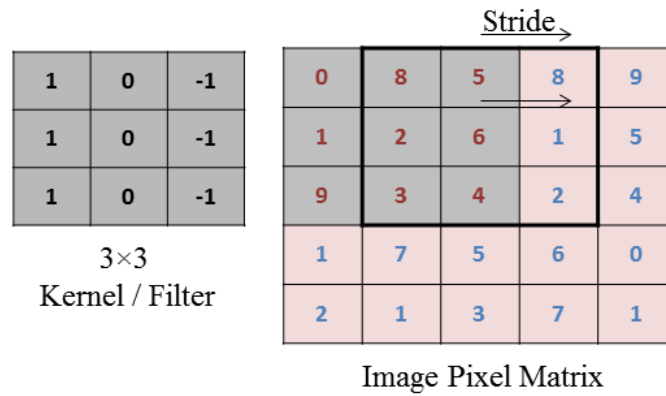
Figure 3.3 Demonstration of sliding window operation, kernel and stride [75].
