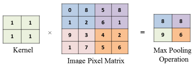
Figure 3.5 Demonstration of max pooling operation using a 2×2 kernel on an image [78].
