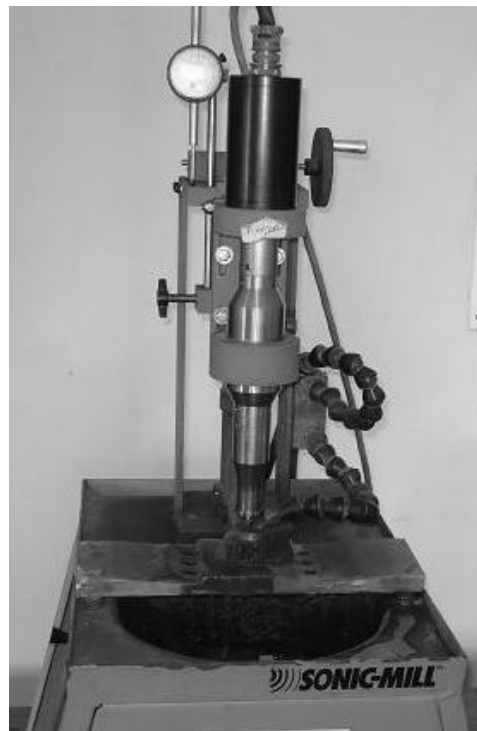
Figure 3.1 Ultrasonic machining Set up [Courtesy by:N.T.M Lab,T.U,Patiala]
