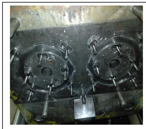
Figure 3.4: Photograph of H13 tool steel die clutch plate (Courtesy: Thapar University, Patiala)
