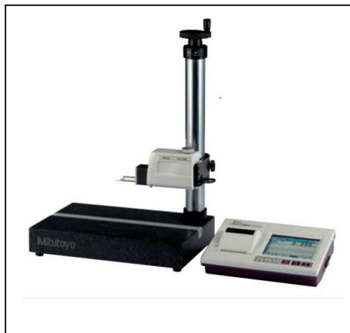
Figure 3.7: Surface Roughness tester Mitutoyo model SJ-400 (Courtesy: Thapar University, Patiala)
