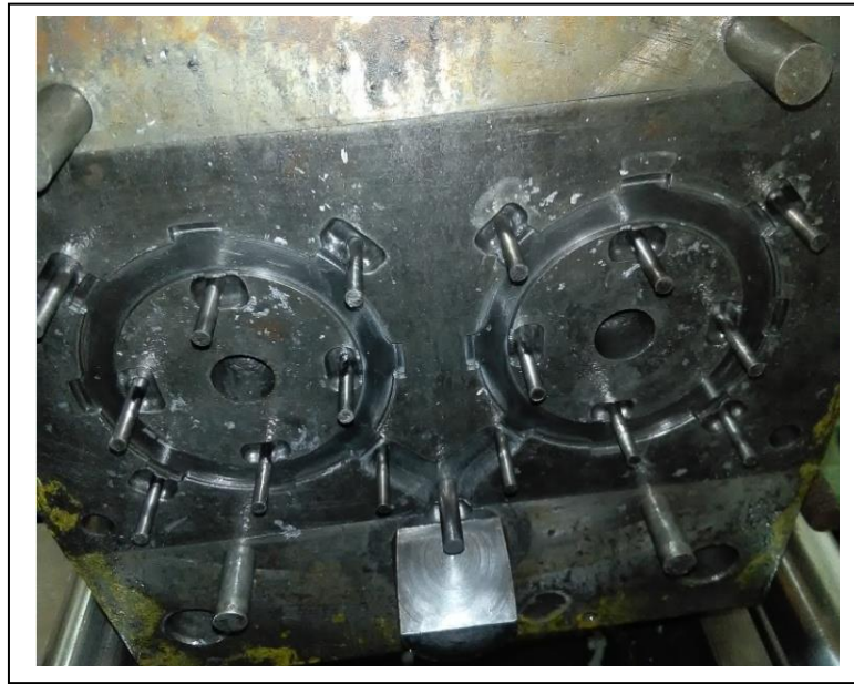
Figure 1.5: Multiple cavity die (clutch plate) at Thapar University
