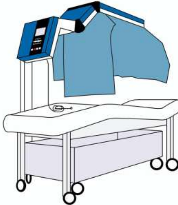
Fig 1.5: Iratherm applicator for whole body hyperthermia (5)
