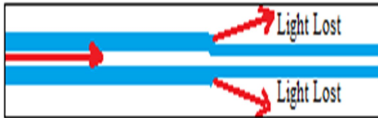
Figure 1.8: Core diameter loss
