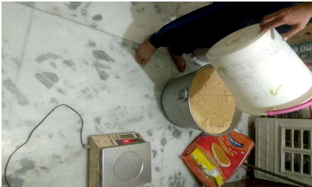
Figure 3.7: Pre-treatment of saw dust with water
