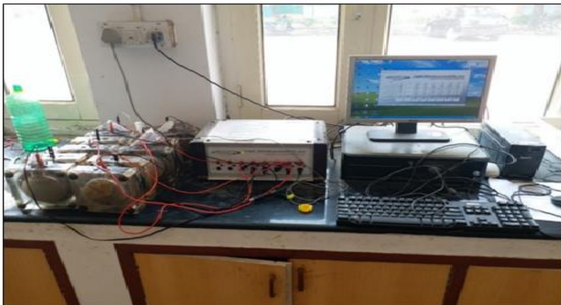
Figure 3.18: Full arrangement of R.C.P.T
