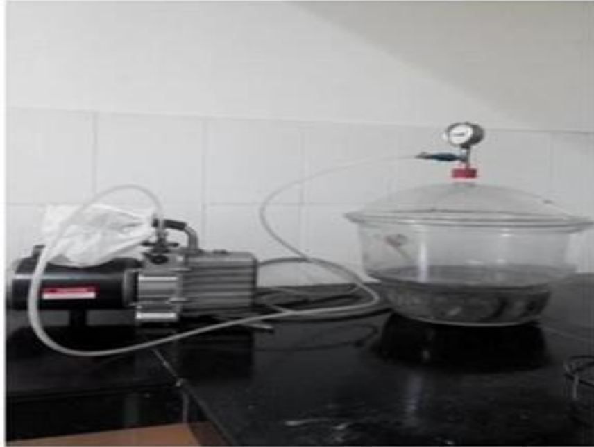
Figure 3.17: Vacuum desiccator bowl
