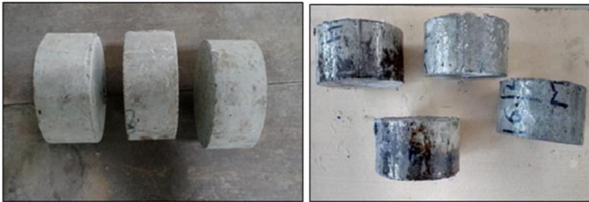
Figure 3.13: 100 mm x 50 mm cylinder A and Epoxy coated sample B
