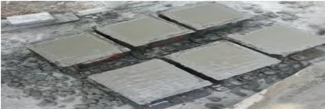
Figure 3.10: Casting of cubes of concrete
