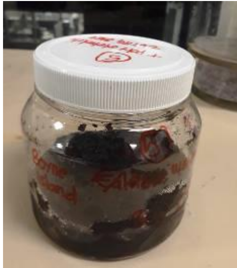
Fig. 4.5 Boyne island WWTP Belt pressed + polyelectrolite zetag 8160
