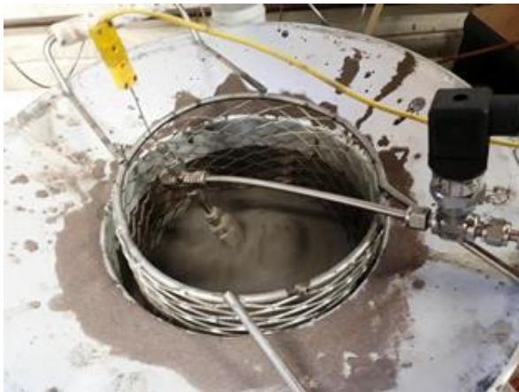
Fig 3.6 HTL reactor heating inside fluidized bath.
