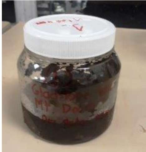
Fig 4.1. Gladstone WWTP dry sludge from dry bed
