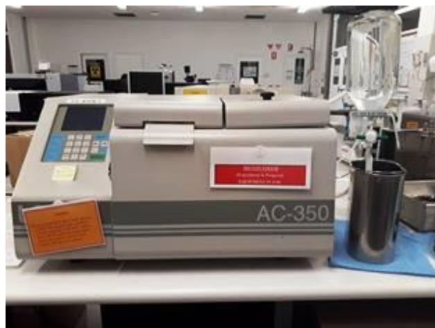
Fig 3.3 Bomb Calorimeter (AC-350)
