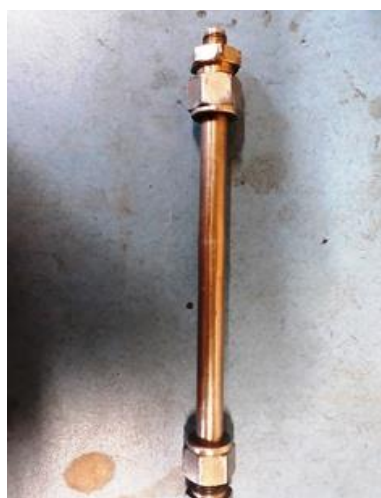
Fig 3.9 5.5 ml reactor for HTL
