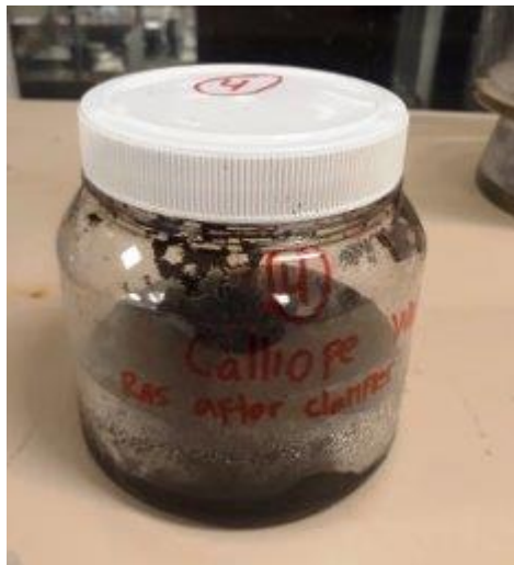
Fig. 4.4 Calliope WWTP RAS after Clarifier QW4: very dark brown slurry , becomes very hard on drying, foul odour.
