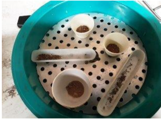
Fig. 3.5 Ash left after heating at 550°C
