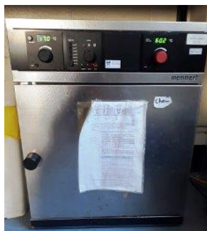
Fig 3.8 oven(40 0 C) to dry the samples
