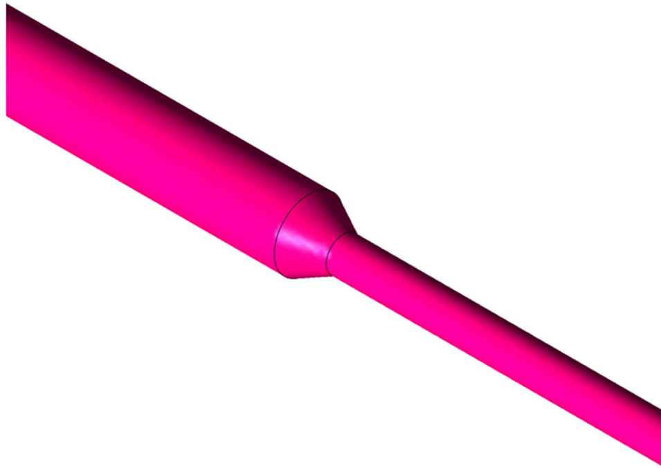
Figure 6.12 Modelled fluid domain for the 0.05m converging section
