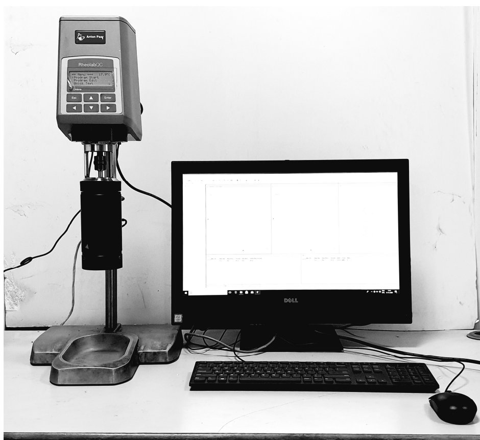
Figure 4.1 RheolabQC rheometer and the attached PC for the data acquisition
