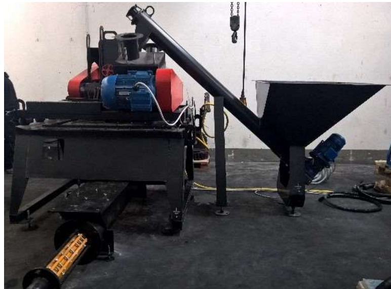
Figure 1.1 A hydroshock machine with a 200litres hopper and a screw conveyor fabricated by DEWA Technologies, Russia. (Source: bit.ly/hrmn13 )
