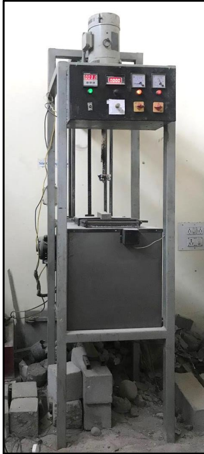
Figure 3.2 Stir casting set-up (Courtesy: TIET, Patiala)
