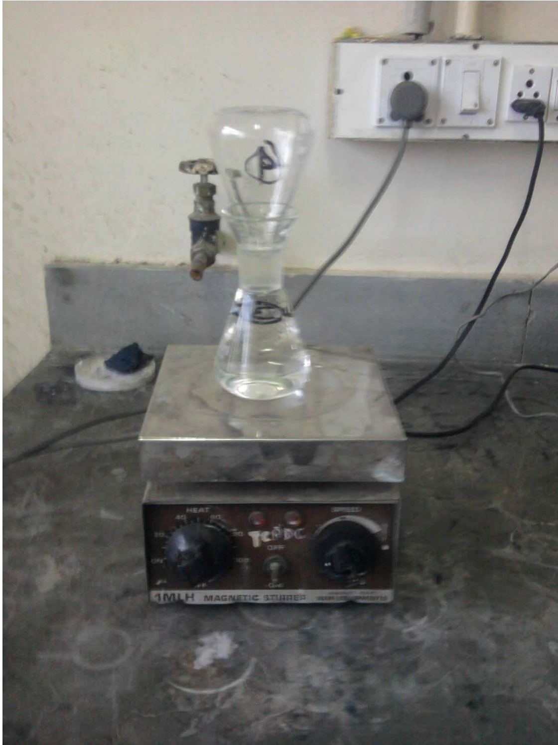
Fig. 6. Headspace BOD experimental setup
