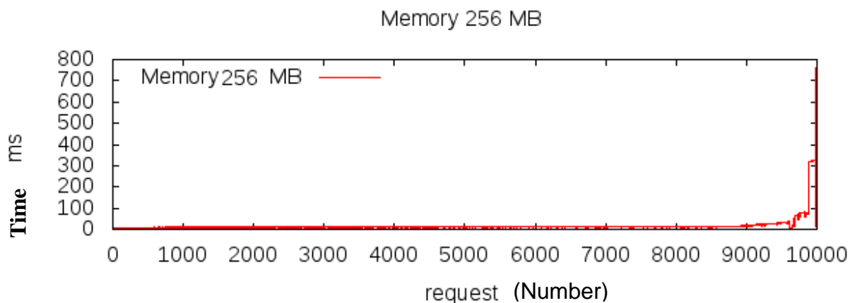
Figure 5.16: Response Time variation on VM with 1 core, 256 MB Memory and traffic load of 10000 requests The graph in Figure 5.17 clearly depicts that how the response time varies when the number of request increases. This machine has configuration of 1 core with 2.53 GHz processor where number of request is 100,000.
