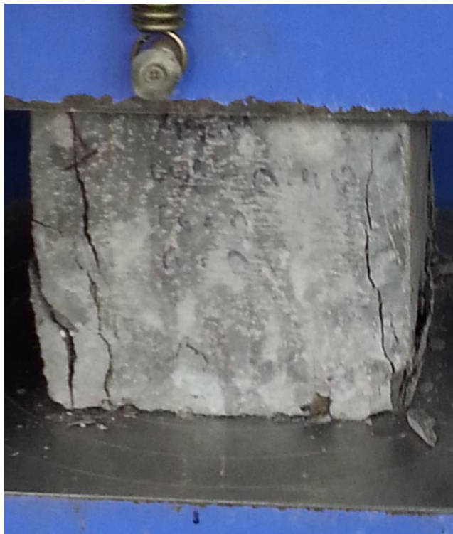
Plate 3.5: Crushed sample during testing.
