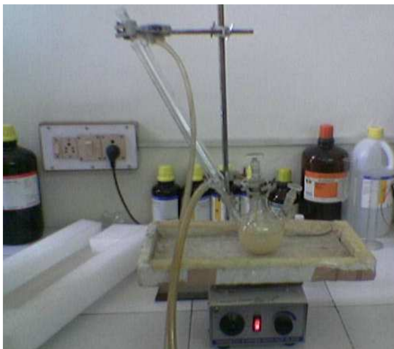
Figure 3.3 Reaction set up used in the lab for synthesis of PANI
