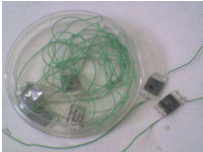
Figure 3.18 Cells with thin film sandwiched between ITO coated glasses
