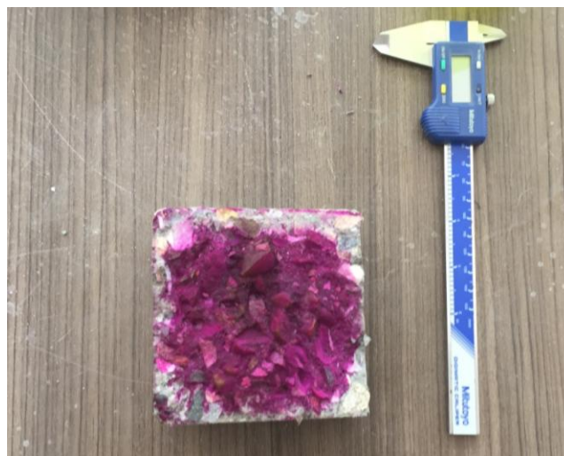
Fig. 5.5: Carbonation depth specimen showing carbonated and non-carbonated part
