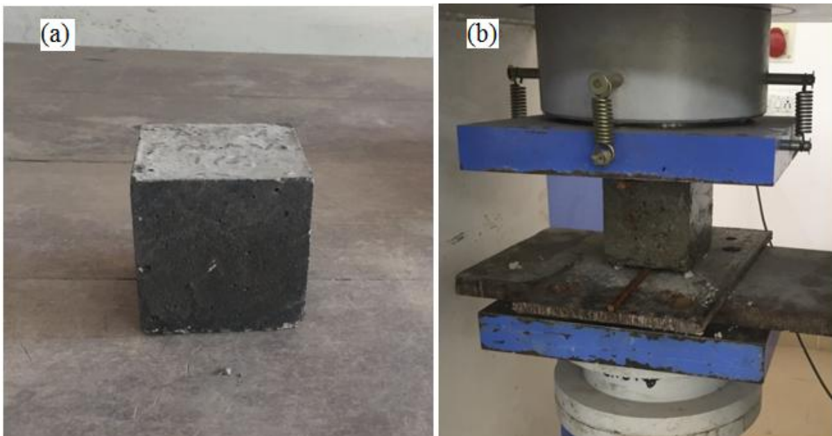
Fig 4.12: (a) Prepared Concrete cube for Carbonation Depth (b) Splitting Concrete Cube into two halves
