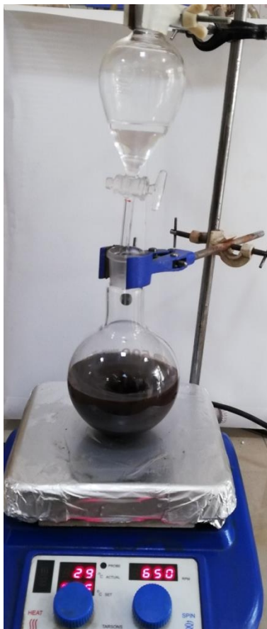
Fig. 7 Preparation of Fe 3 O 4 @SiO 2 MNPs
