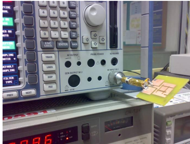
Fig. 3.21 Photograph of Prototype Antenna
