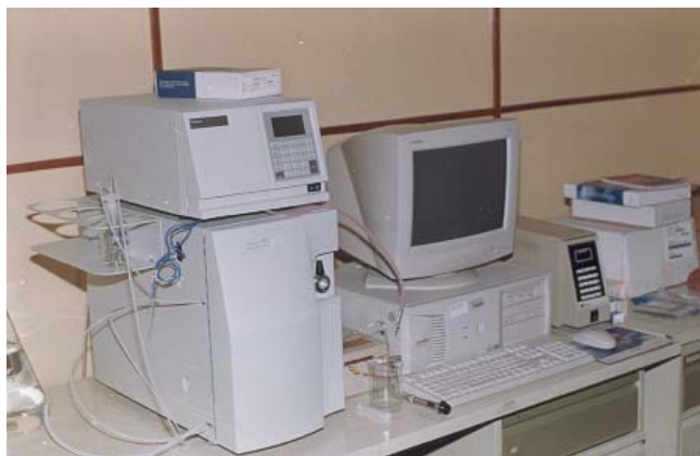
Fig.2.14 Furfuraldehyde analysis set up
