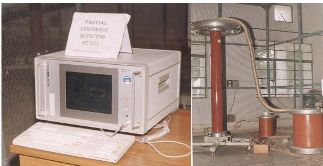
Fig. 2.18 Partial Discharge measurement set up
