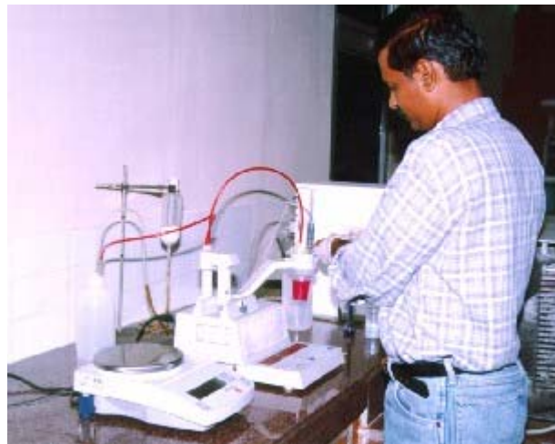
Fig.2.10 Acidity measurement Set up
