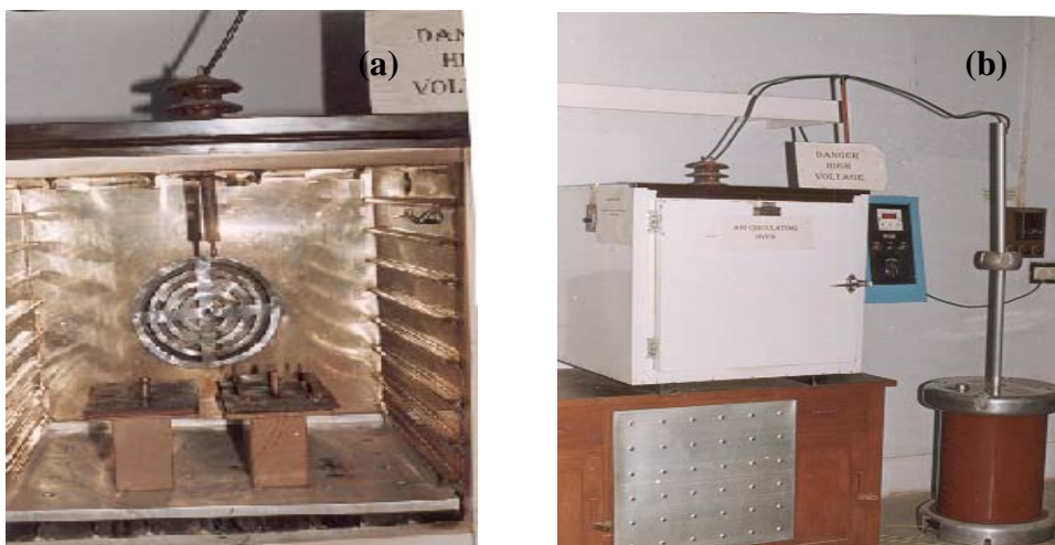
Fig. 2.4 Thermal and electrical aging set up
