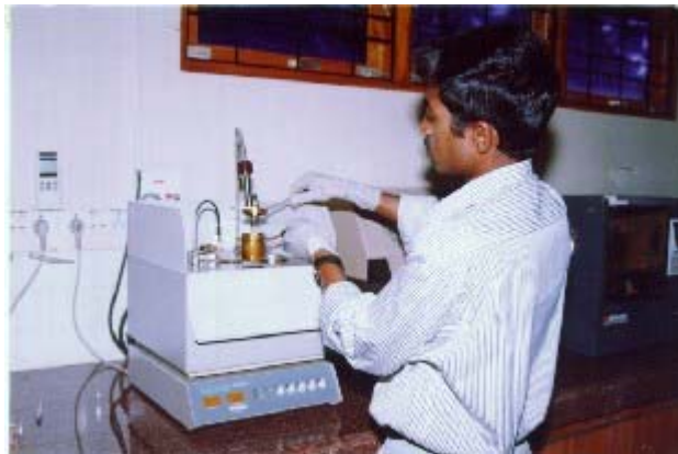
Fig.2.11 Flash Point measurement set up
