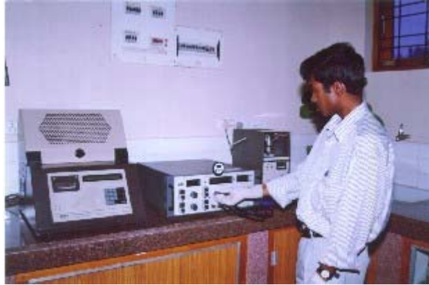
Fig. 2.9 Specific resistance set up
