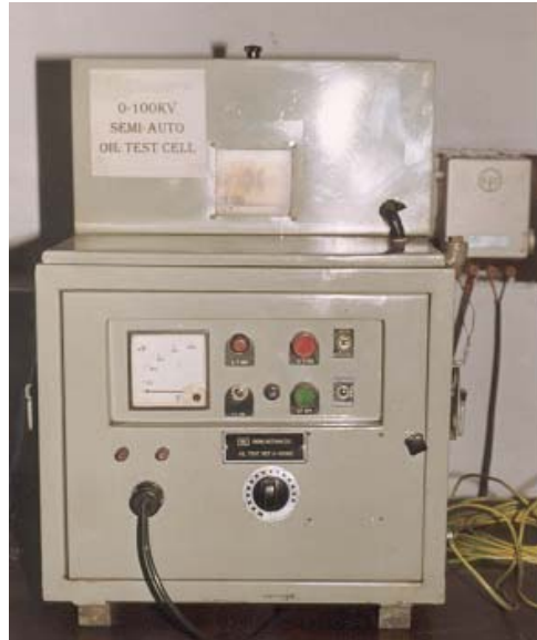
Fig. 2.6 BDV set up
