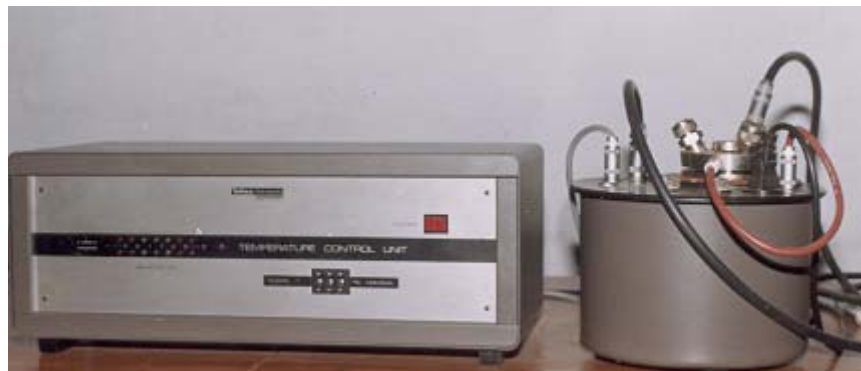
Fig. 2.7 Tan-delta set up
