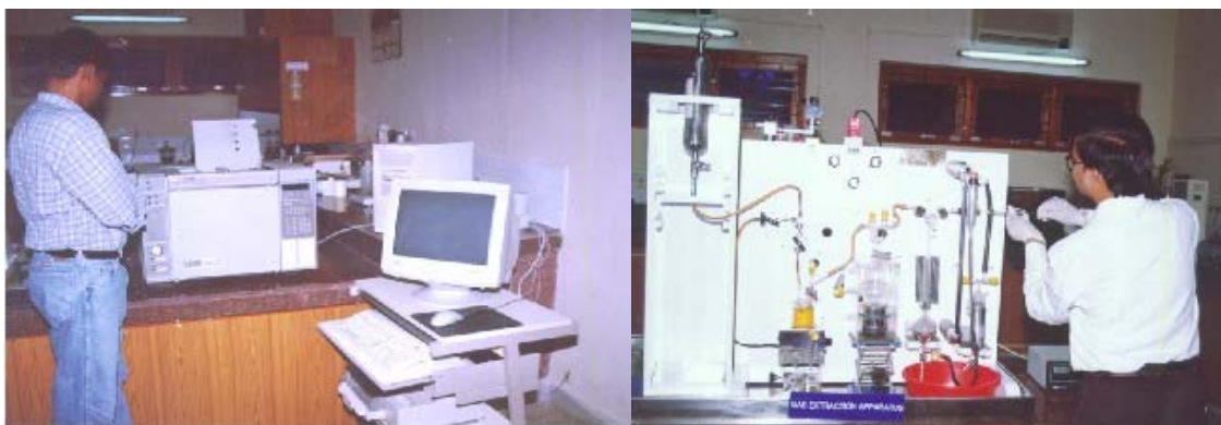
Fig. 2.13 Dissolved gas analysis set up
