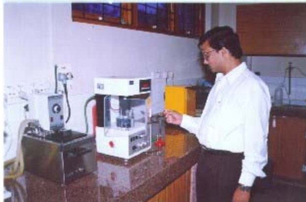
Fig. 2.8 Interfacial tension set up
