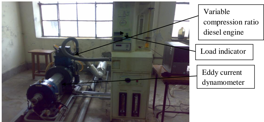
Plate 3.5. Variable compression diesel engine
