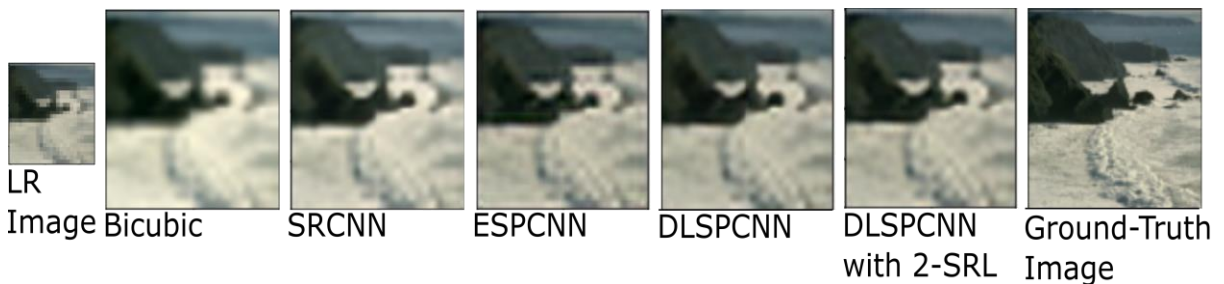
Figure 6.2 SR results. The ‘117025’ image from the B500 is upscaled by the factor of 4 using different state-of-the art algorithms.
