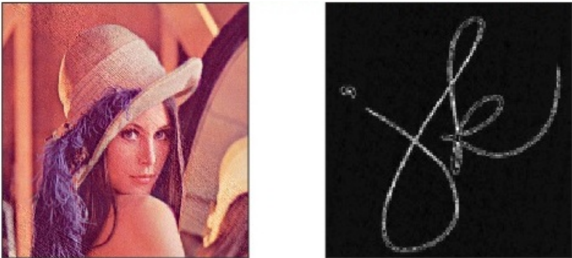
Figure 5.18: (a) Watermarked image after Sharpening (b) Extracted Watermark after applying Sharpening Attack when Ridgelet Transform is used for decomposition
