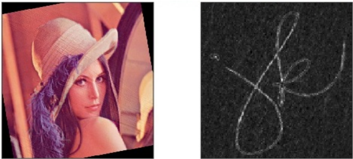
Figure 5.14: (a) Watermarked image after Rotation (b) Extracted Watermark after applying Rotation Attack when Ridgelet Transform is used for decomposition
