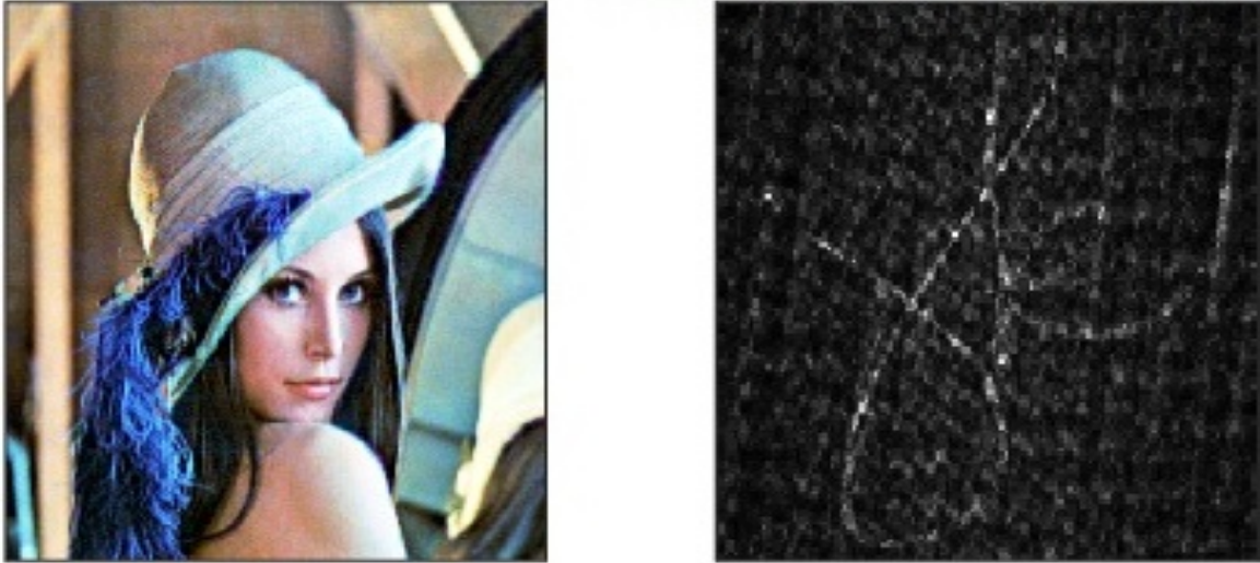
Figure 5.9: (a) Watermarked image after Histogram Attack (b) Extracted Watermark after applying Histogram Attack when Curvelet Transform is used for decomposition
