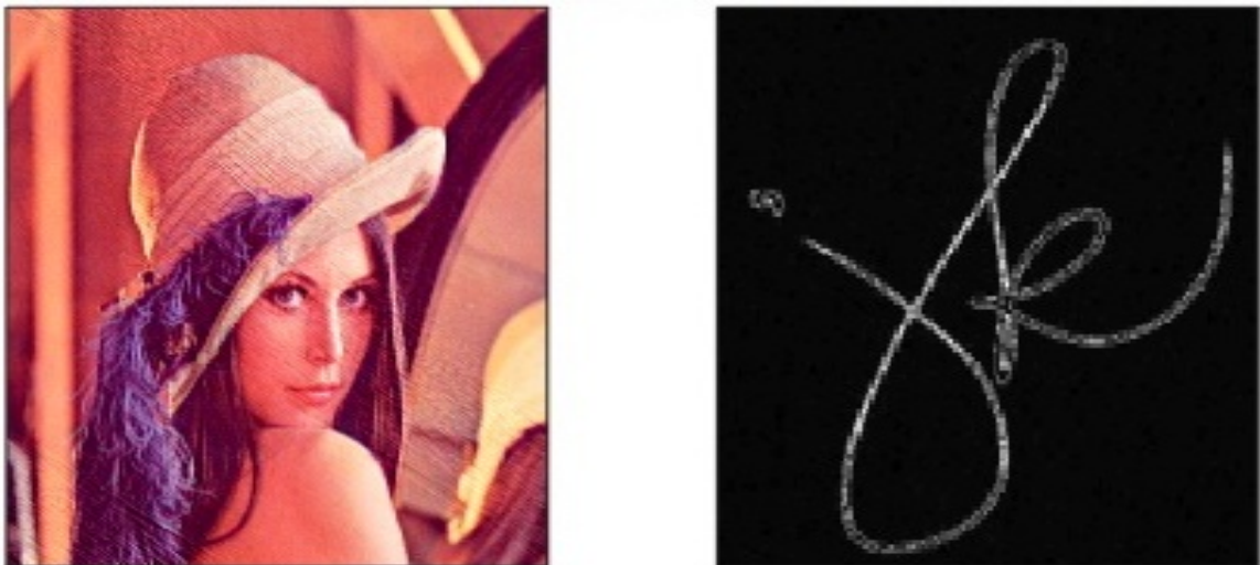
Figure 5.6: (a) Watermarked image after Contrast Enhancement (b) Extracted Watermark after applying Contrast Enhancement attack on RT
