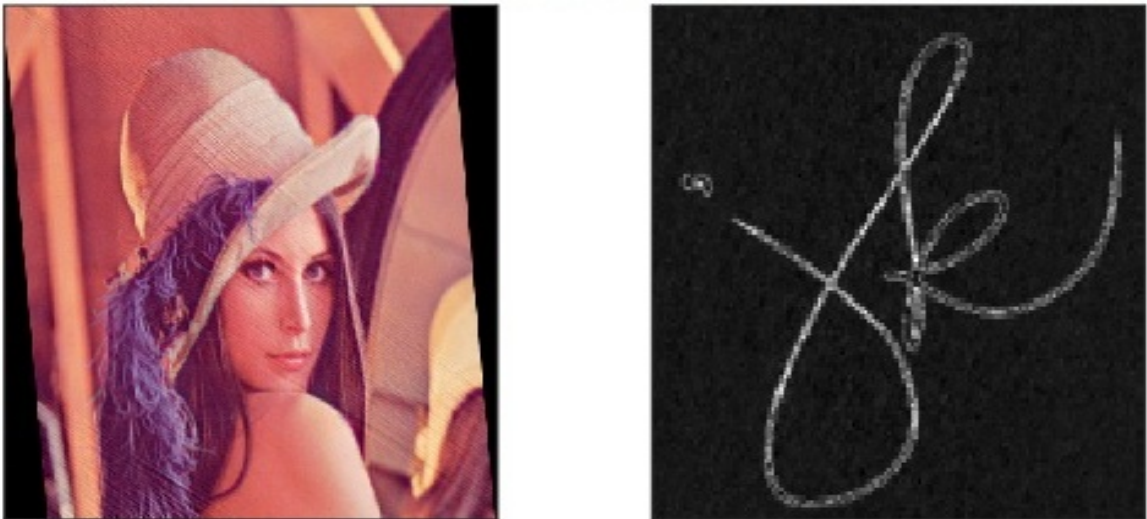
Figure 5.20: (a) Watermarked image after X-Shear (b) Extracted Watermark after applying X-Shear Attack when Ridgelet Transform is used for decomposition
