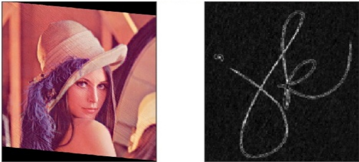
Figure 5.22: (a) Watermarked image after Y-Shear (b) Extracted Watermark after applying Y-Shear Attack when Ridgelet Transform is used for decomposition
