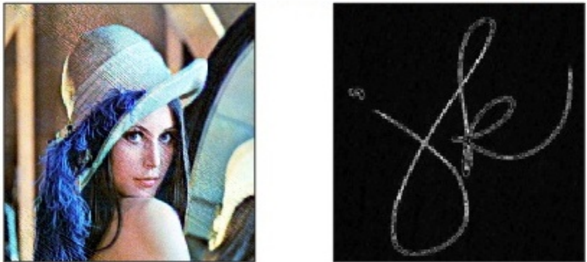
Figure 5.10: (a) Watermarked image after Histogram Attack (b) Extracted Watermark after applying Histogram Attack when Ridgelet Transform is used for decomposition
