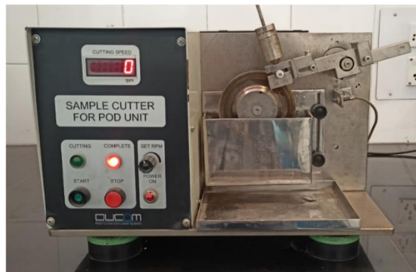
Figure 3.7 Precision cutter (Courtesy: Thapar Institute of Engineering and Technology, Patiala).
