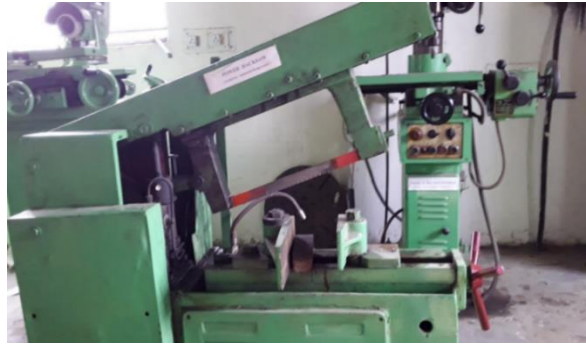
Figure 3.2 Power hacksaw machine (Courtesy: Thapar Institute of Engineering & Technology, Patiala).
