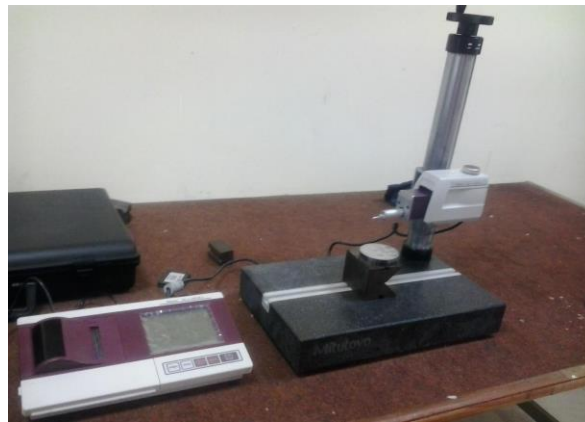
Figure 3.14 Surface roughness tester (Courtesy: Metrology Lab, Thapar Institute of Engineering and Technology, Patiala).
