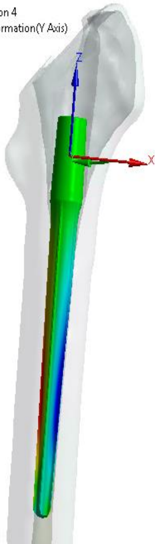
Figure 5.14: Rotational Deformation for Assembly Load in AP (L) and ML (R) view. (Workbench)
