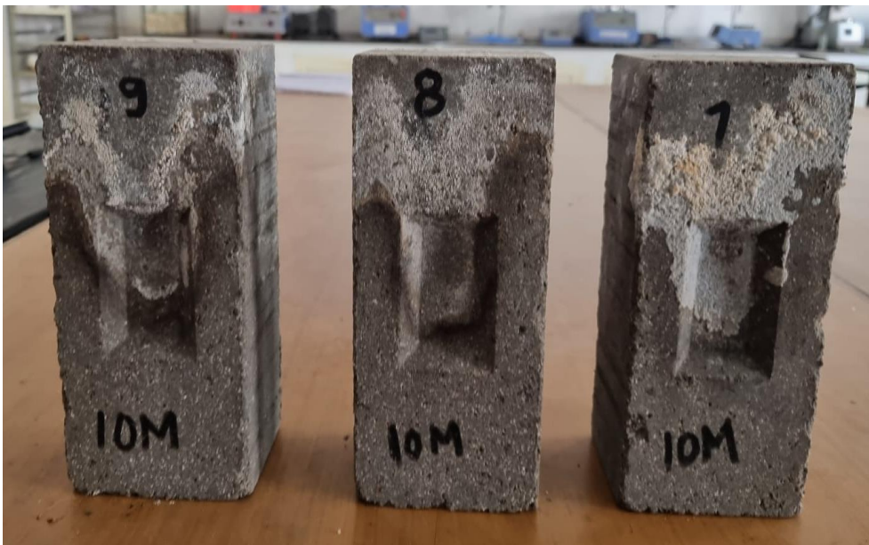
Figure 4.11 Formation of salts layer on front face
