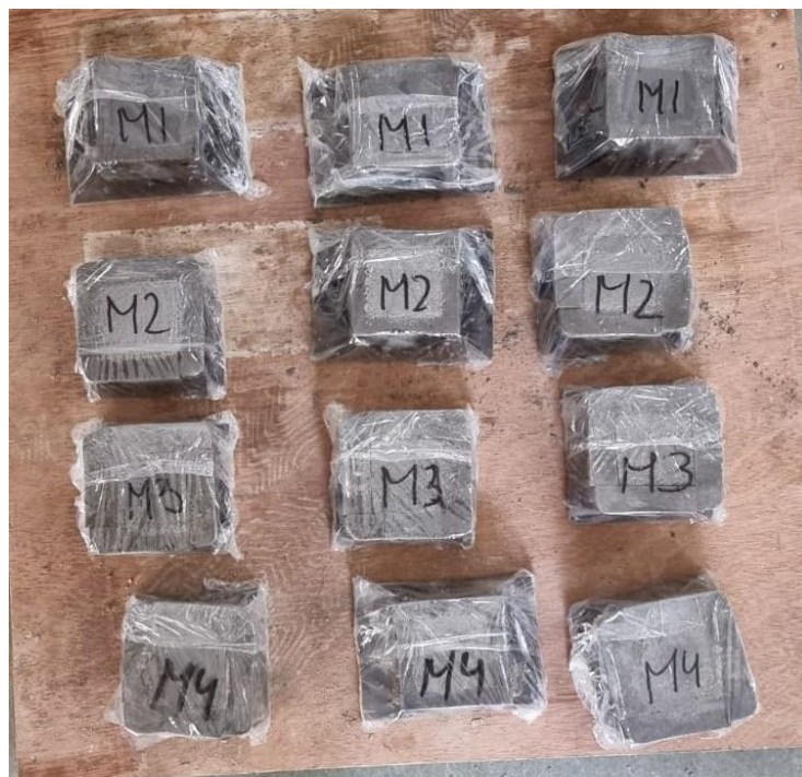
Figure 3.18: Mould wrapped with a thin film of plastic polythene
