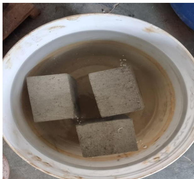
Figure 3.39: Bricks immersed in water (18M) for 24 hours
