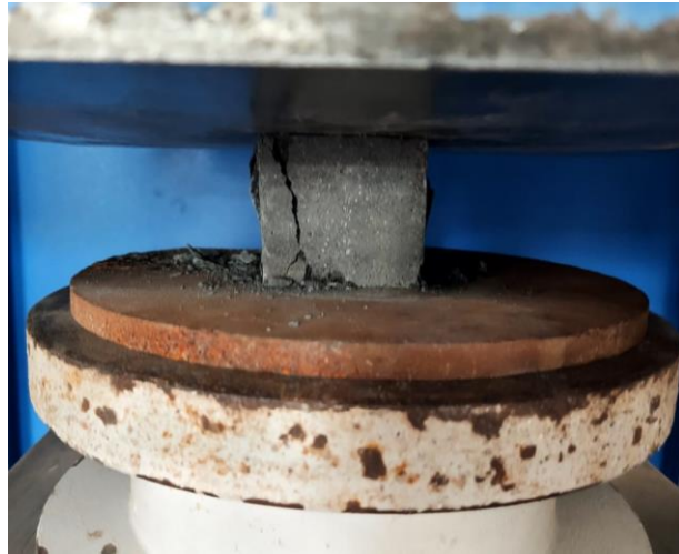
Figure 3.31: CTM for compressive strength test
