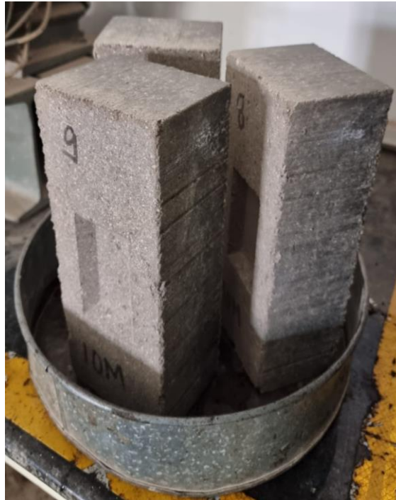
Figure 3.40: 10M bricks placed in the pan
