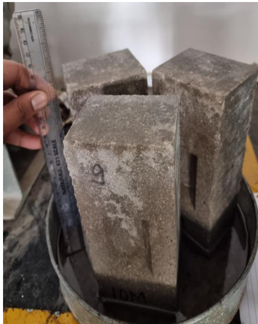
Figure 3.44: Bricks submerged in distilled water (25mm)
