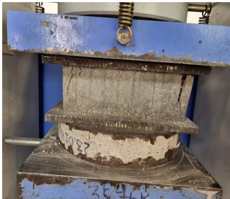
Figure 3.35: Failure of the brick in CTM
