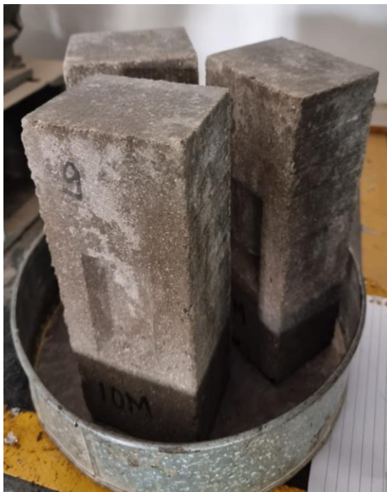
Figure 3.43: Bricks completely absorbed the distilled water after 1 day
