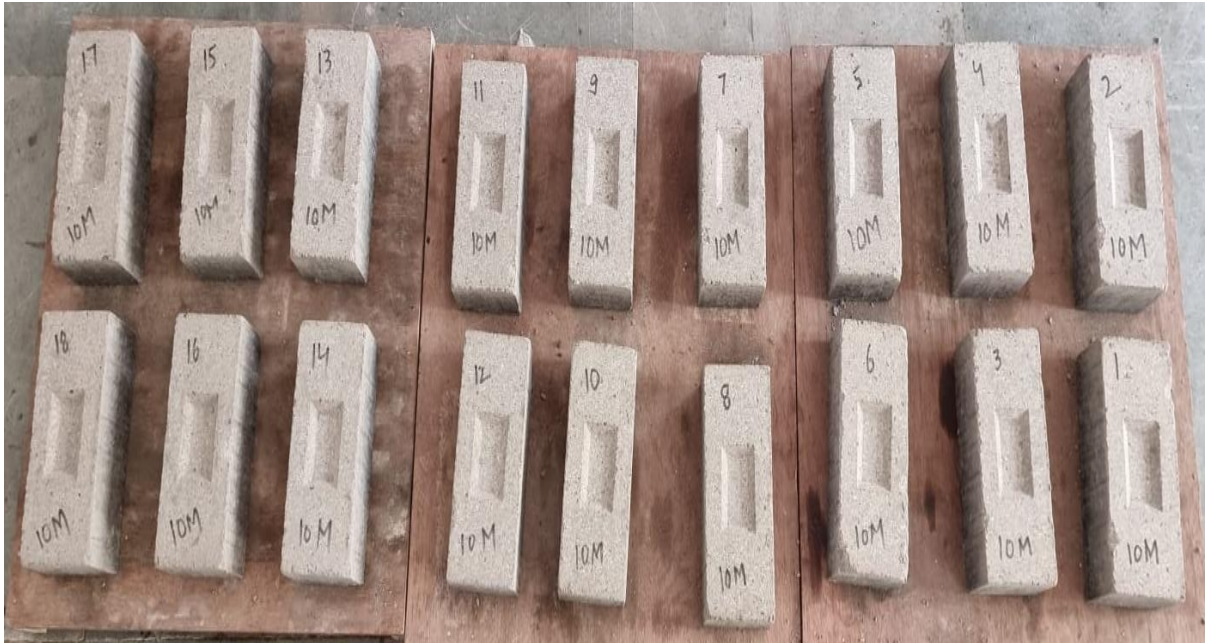
Figure 3.28: Casted bricks (10M)
