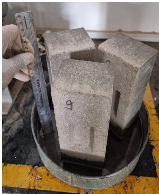
Figure 3.41: Bricks submerged in distilled water (25mm)
