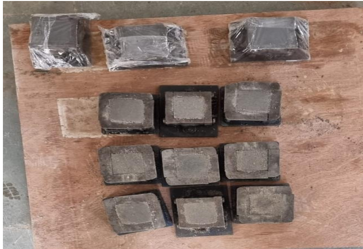
Figure 3.17: Casting of the cubical moulds
