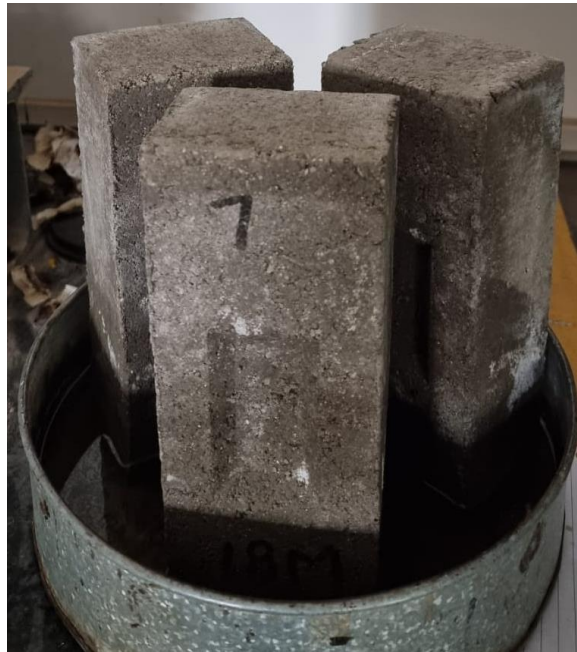
Figure 3.47: Bricks submerged in distilled water after 2 days
