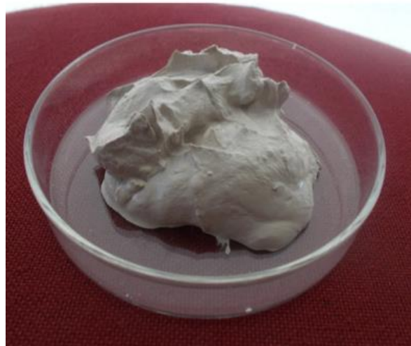
Figure 1.2: Brine sludge as obtained from a chlor-alkali plant (Joshi et al. 2015)
