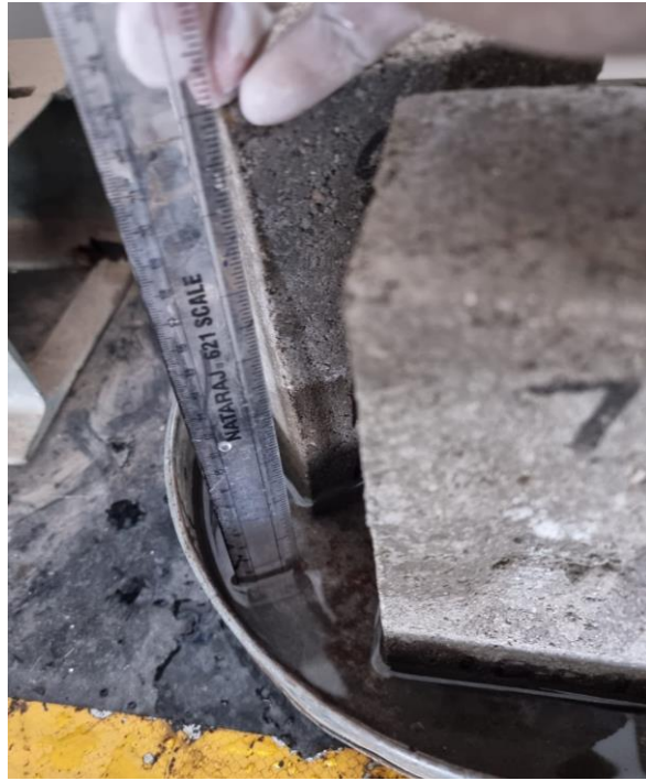
Figure 3.46: Bricks submerged in distilled water (25mm)
