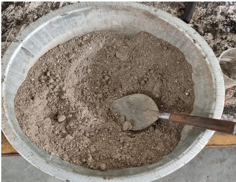
Figure 3.23: Wet mix in head pan
