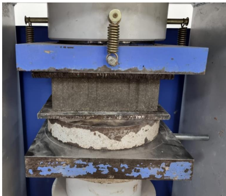
Figure 3.37: Brick placed in CTM
