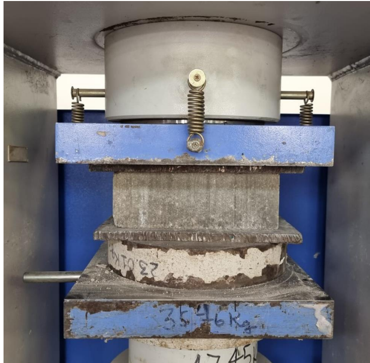
Figure 3.34: Brick placed in CTM
