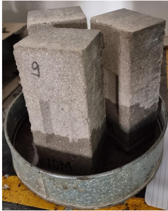
Figure 3.42: Bricks submerged in distilled water after 2 hours
