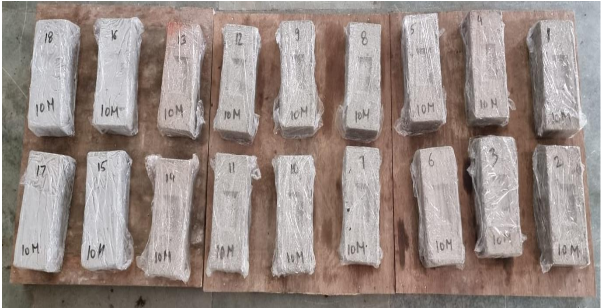
Figure 3.26: Bricks wrapped with a thin film of plastic polythene (10M)
