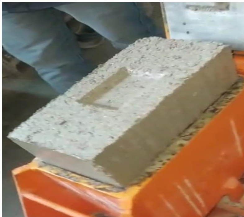
Figure 3.25: Demoulding of brick
