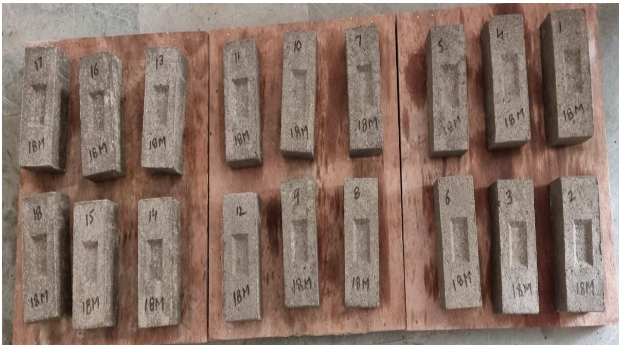
Figure 3.29: Casted bricks (18M)
