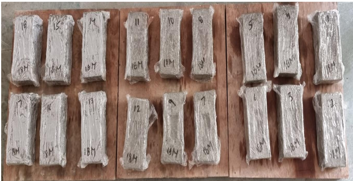
Figure 3.27: Bricks wrapped with a thin film of plastic polythene (18M)
