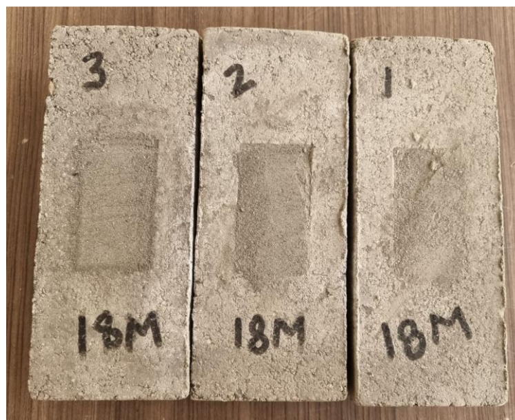
Figure 3.33: Bricks (18M) for compressive strength test
