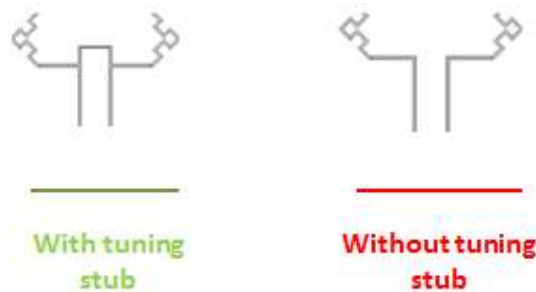
Fig.3.3 (b) Antenna with and without tuning stub
