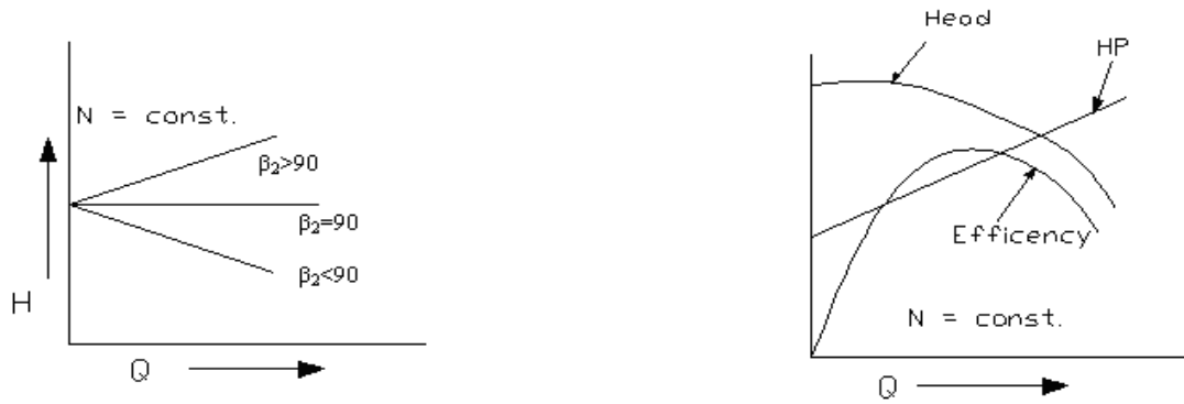
Figure 1.11 Operating characteristic curves of centrifugal pump
