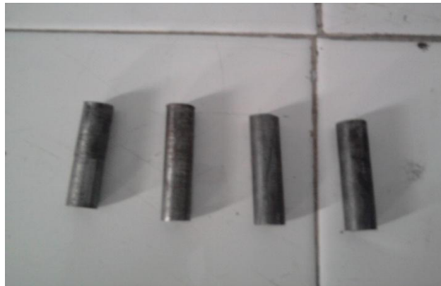
Fig. 4.14 Pins Used for Wear Test
