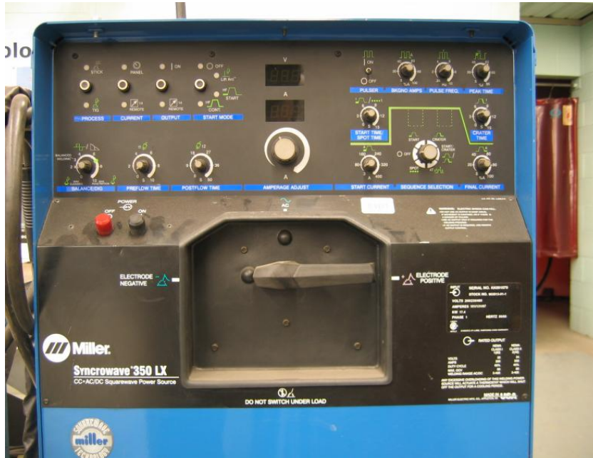
Fig. 1.4 High Output Welding Power Supply for SMAW [1]
