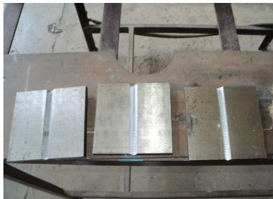
Fig. 4.6 Plates after Machining on Shaper
