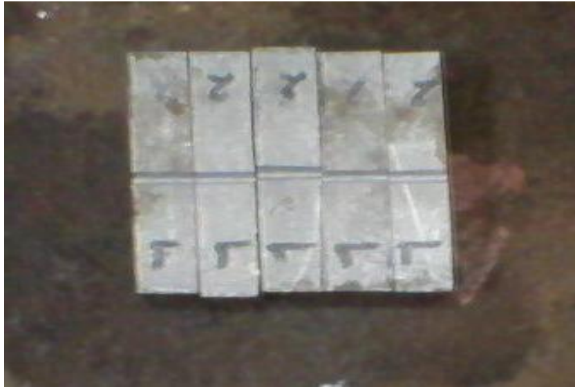
Fig. 4.12 Specimens Made for Impact Testing
