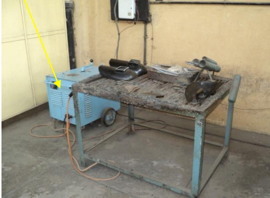
Fig. 4.7 Complete Set Up of MMAW Machine
