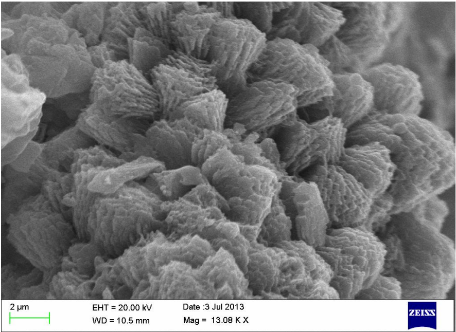
Fig 4.11 (b) Close View of the Cement Mortar at point 12 with Fungus #21 CMSTITNEY ( 2 μm)
