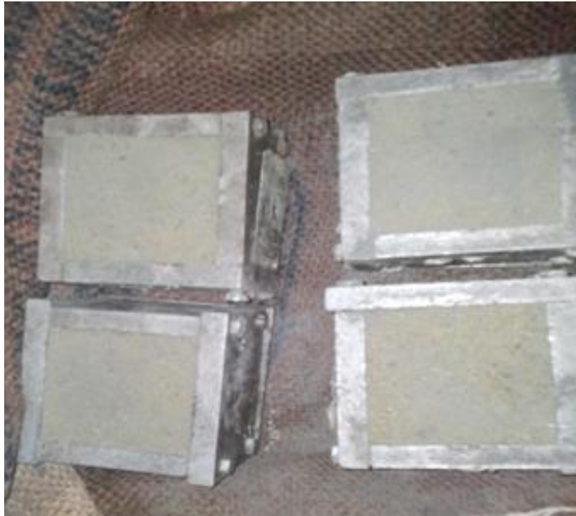
Fig. 4.7 (a) Controlled Mix Cubes in Moulds
