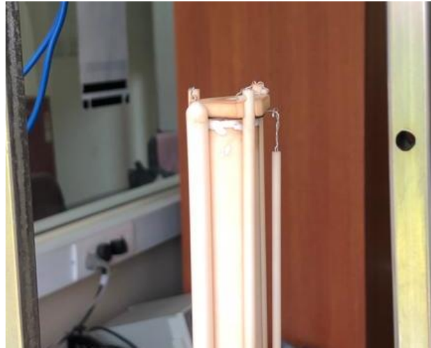
Fig 3.9 SOFC button cell mounted on the sample holder and sealed using silver rings and silver paint
