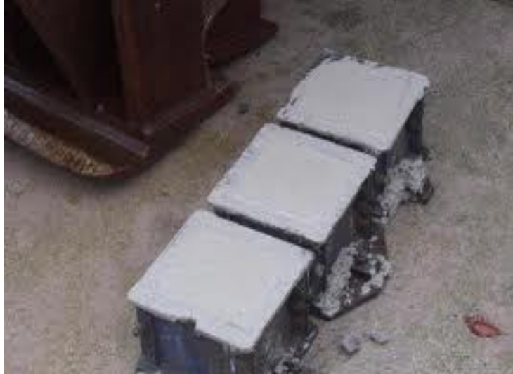
Figure 3.3: Casting of cubes
