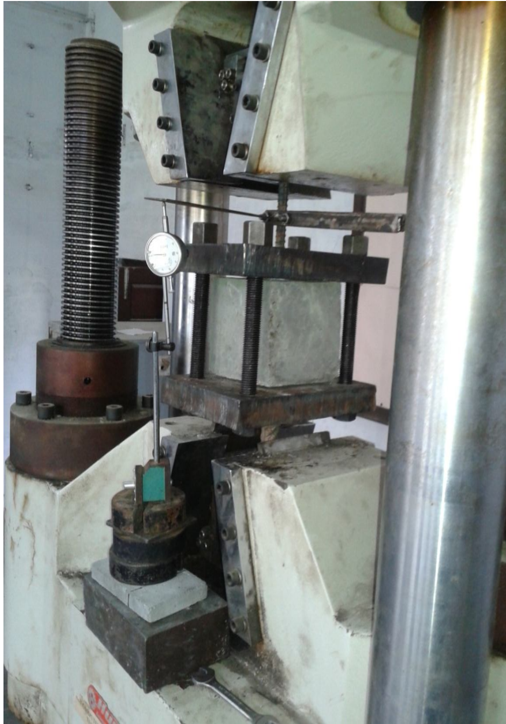
Figure 3.8: Test setup for pull out strength test
