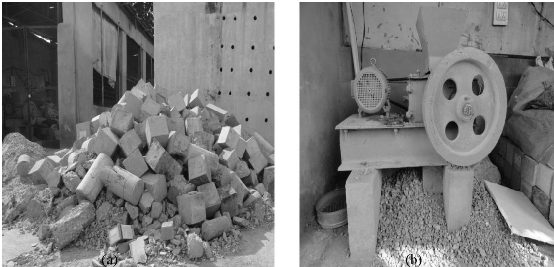
Figure 3.1: (a) Waste concrete used for producing RCA (b) RCA obtained from the jawcrusher
