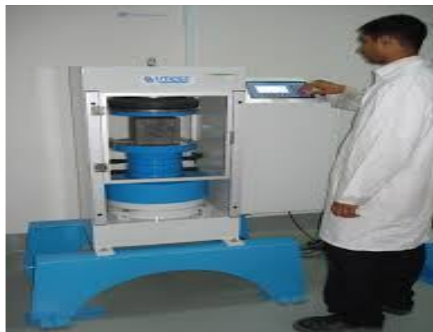
Figure 3.6: Compressive strength test machine
