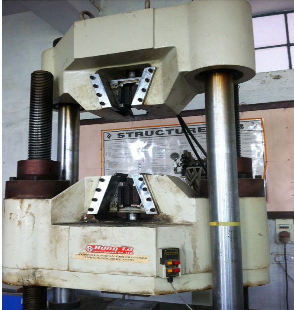
Figure 3.7: Pull out test machine
