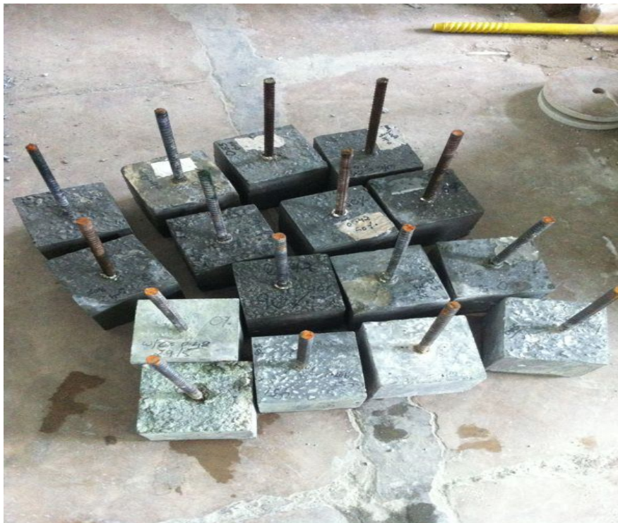
Figure 3.4: Pull out test concrete specimens
