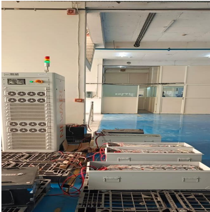
Fig.8 Charging and Discharging Testing By Machine
