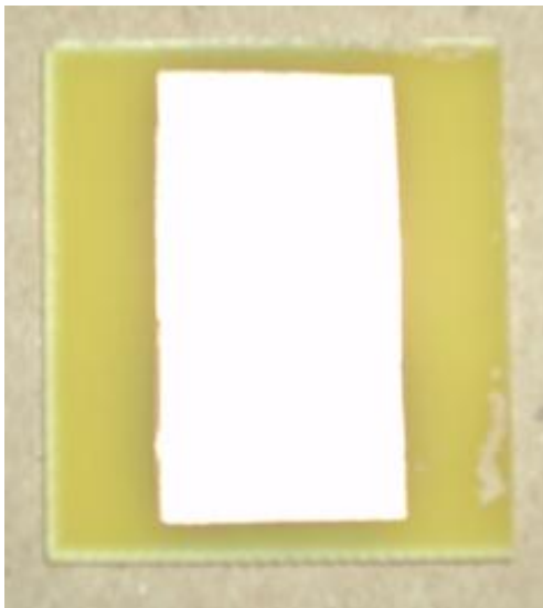
(a) Top view of Antenna showing Patch
