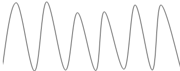
Figure-2.1: Voltage Sag
