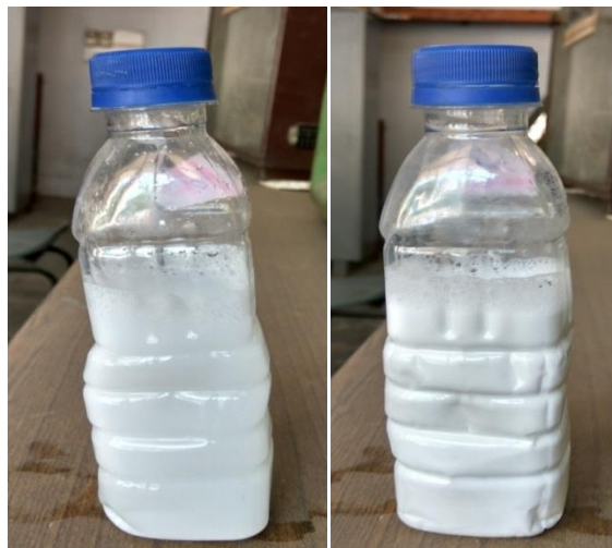
Figure 1.3: \text{Al}_2\text{O}_3 nanofluid solution a) without surfactant b) with surfactant.
