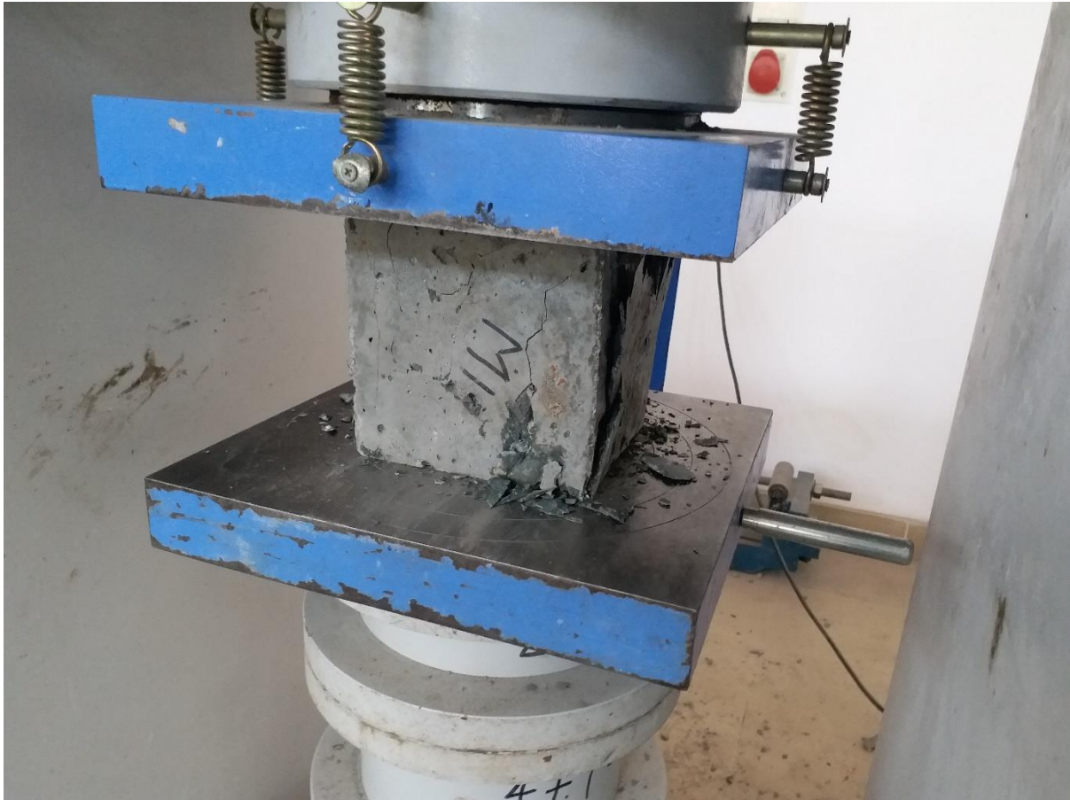
Fig.3.6: Cube after compression test in Automatic Compression Testing Machine (ACTM)
