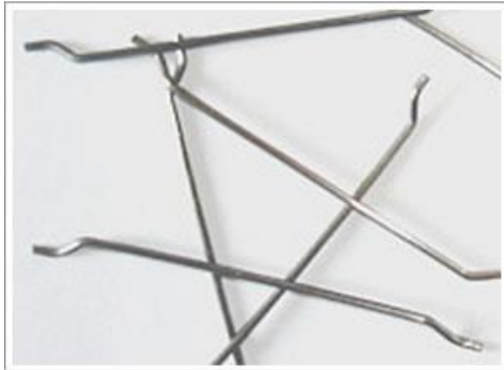
Fig.1.6: Hooked steel fibers (Source: www.steelfiber.org )
