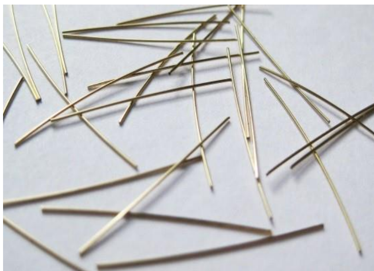
Fig.1.5: Straight steel fibers (Source: www.steelfiber.org )
