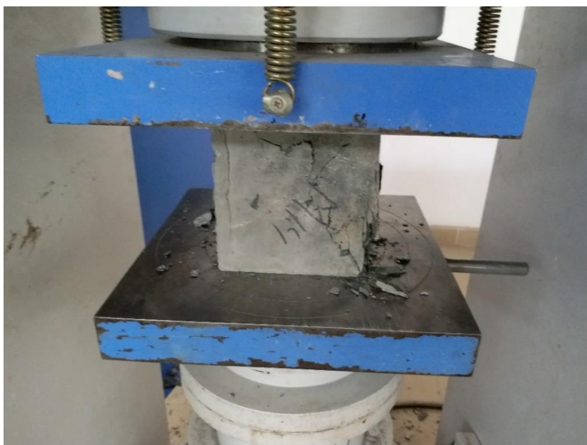
Fig.4.10: Specimen under sulphate attack in ACTM
