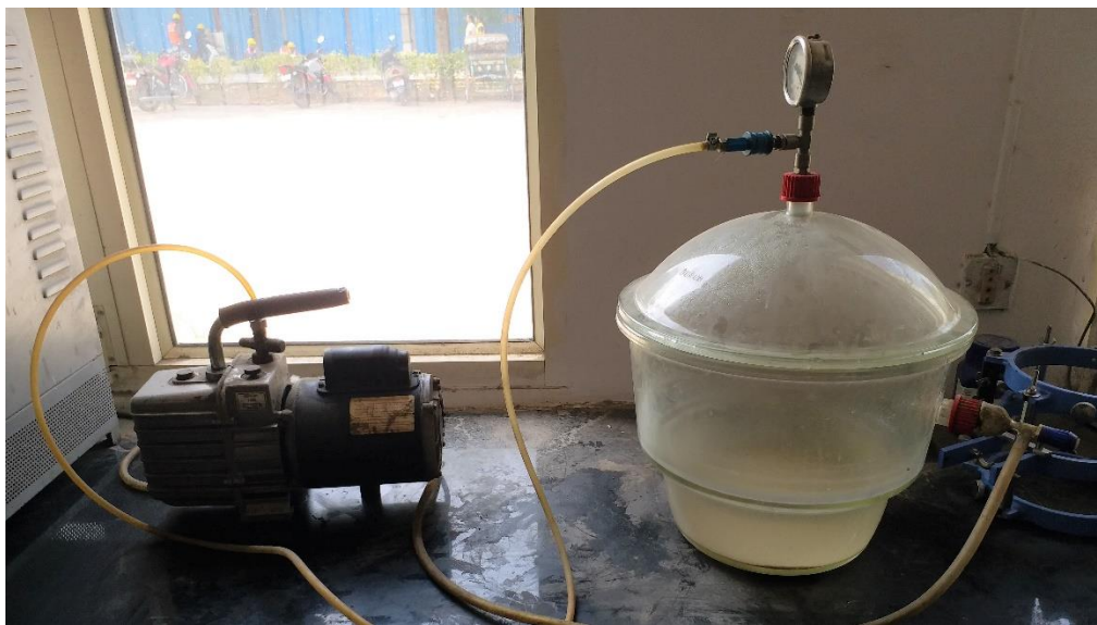
Fig.3.8: Vacuum desiccators' bowl
