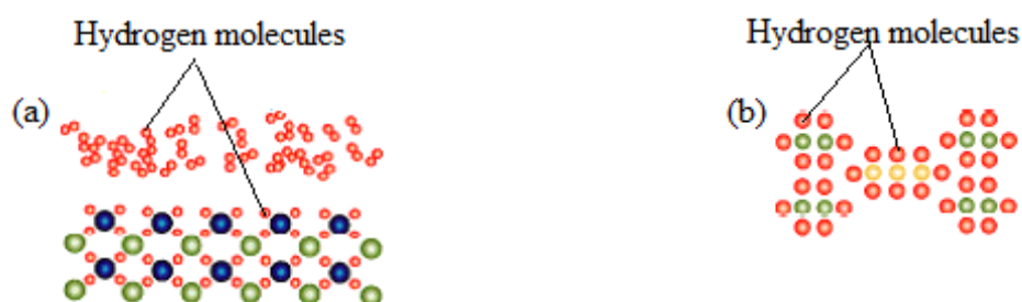
Figure 1.4 (a & b): Absorption of hydrogen molecules in complex chemical hydrides (Klanchar and Lloyd, 2000)
