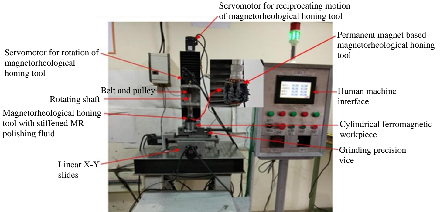
Fig. 1.12 Photograph of the experimental setup of the magnetorheological honing process for finishing the internal surface of variable diametric cylindrical workpieces (Grover and Singh, 2018).
