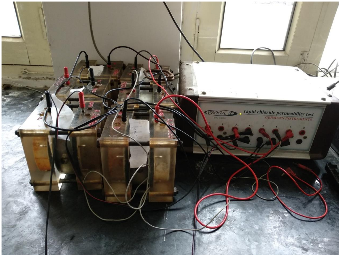
Fig 3.4: Rapid chloride permeability test
