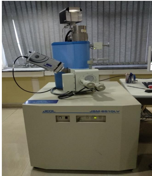
Fig 3.7: Scanning electron microscope (SEM)
