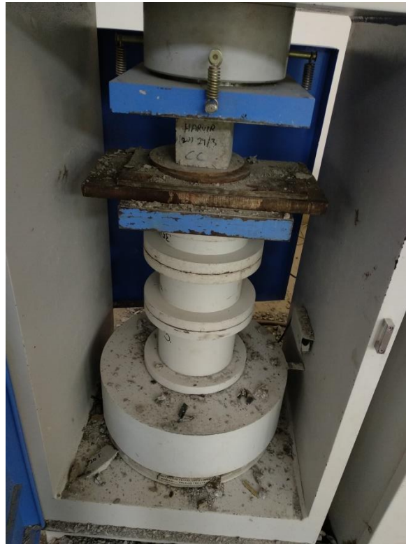
Fig 3.3: Compression testing of cubes
