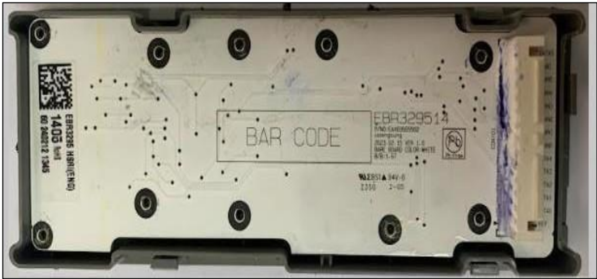
Fig 4.2 ThinQ Display Back Panel
