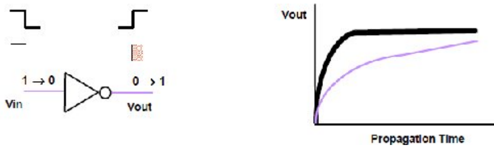
Figure 2.8 Logic example depicting transition delay
