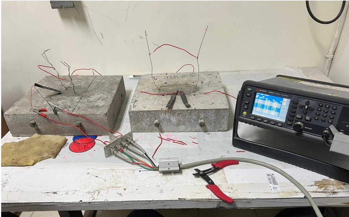
Figure 3. 17 Health monitoring of anode through LCR meter
