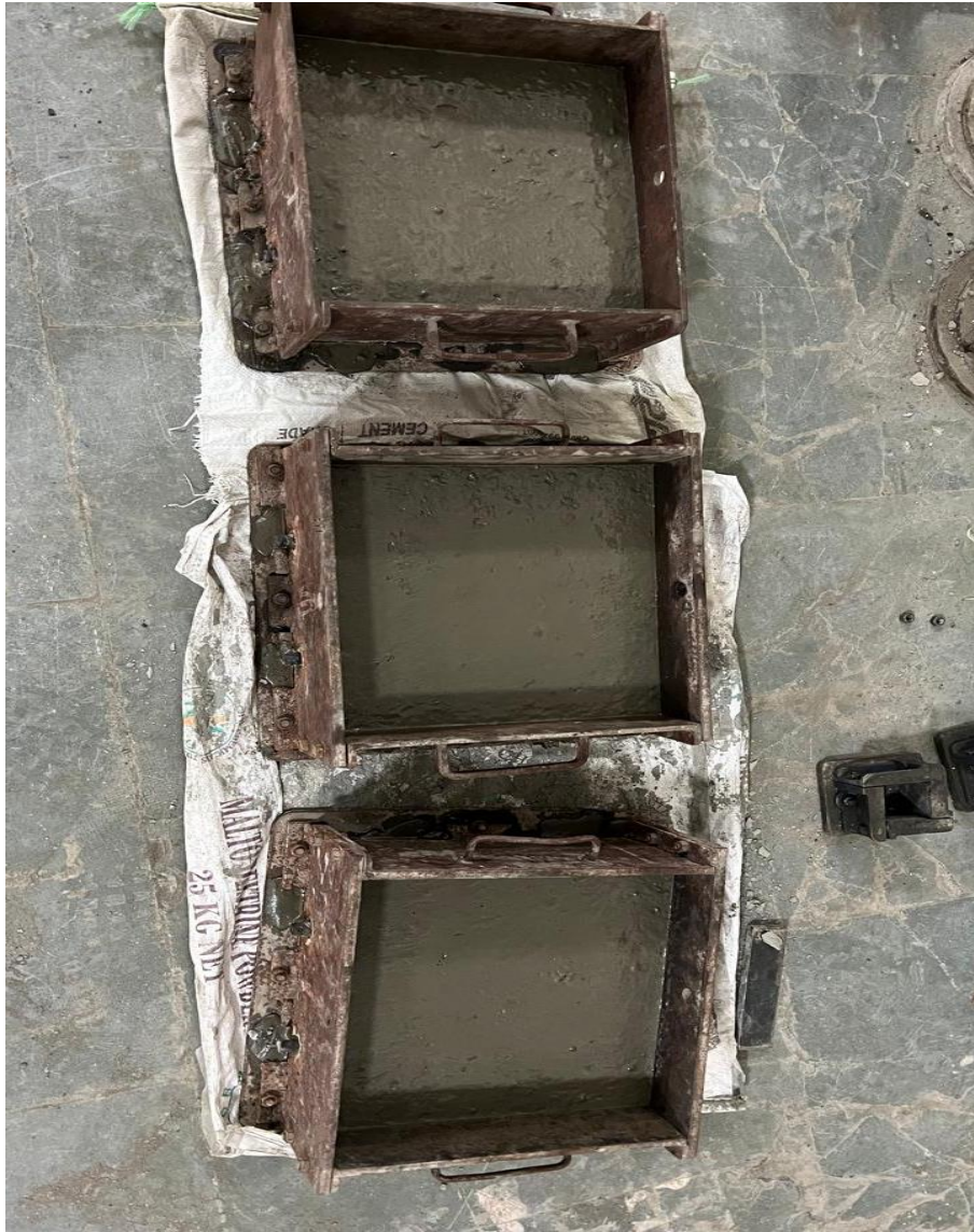
Figure 3. 11 Concrete M40 was filled upto 80mm
