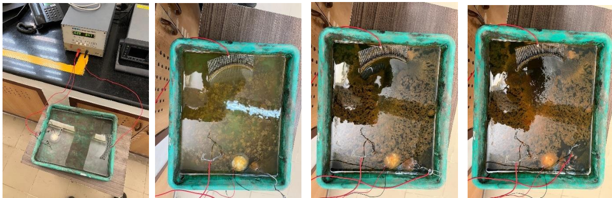
Figure 4. 15 Progressive change in color of electrolyte due to corrosion of the sacrificial (Anode A)
