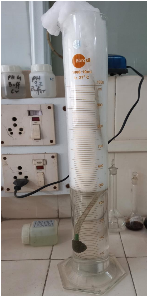
Figure 7.4: Foam formation after aeration for 1.5 minutes
