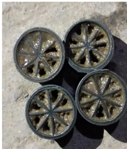
Figure 4.3: Biological growth in the carrier media
