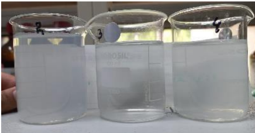
Figure 7.3: Supernatant of jar test 2, 3 and 4
