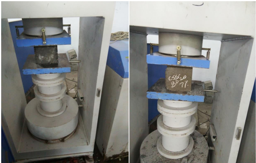
Plate 3.4: Testing of Cube for compressive strength on ACTM
