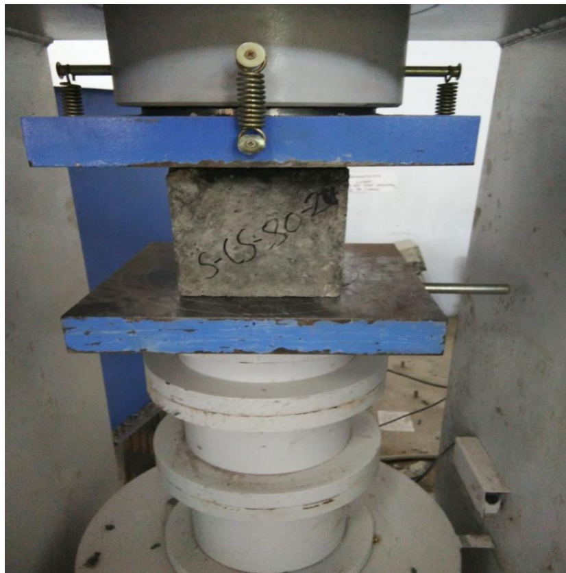
Plate 3.3: Testing of Cube for compressive strength
