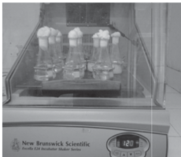
Fig. 2. Shaker incubator used for degradation experiments
