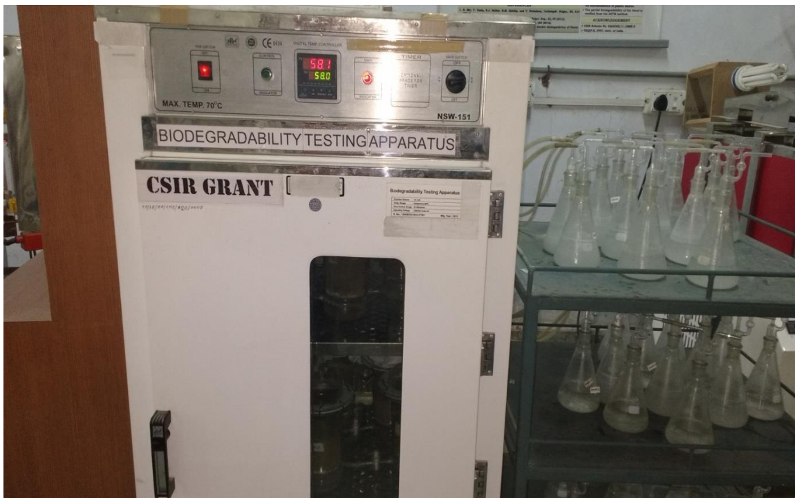
Figure 3.6 Biodegradability testing apparatus for determining percentage biodegradation
