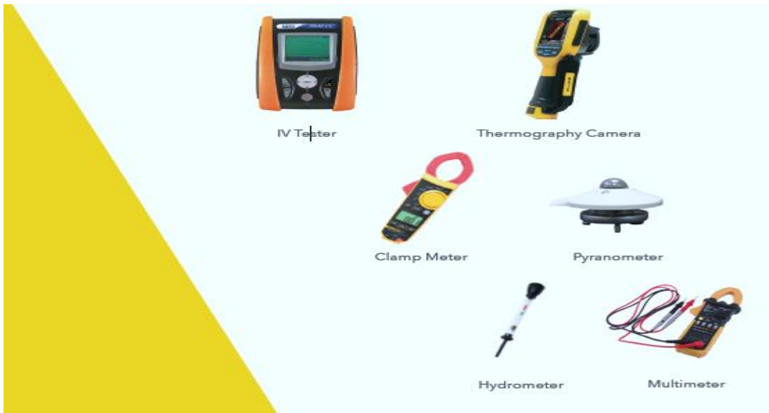
Fig. 5.1 Equipment used in the maintenance for solar plant
