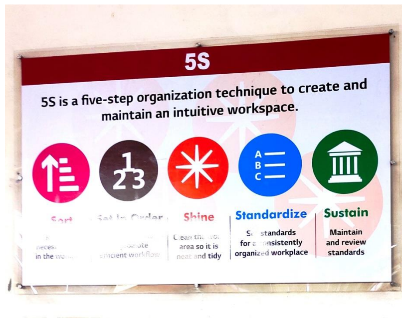
Fig. 4.4 a 5S hoarding at the factory premises
