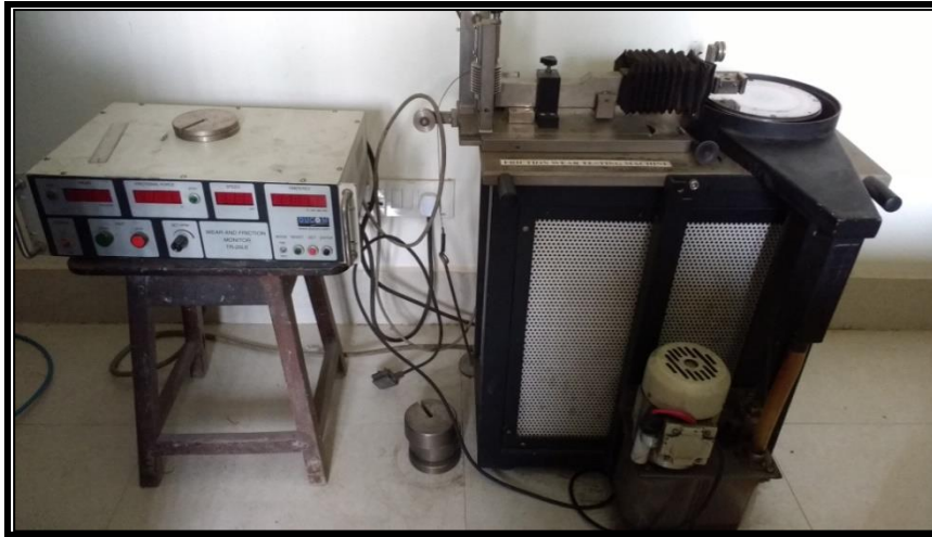
Figure 3.2: Wear testing setup (Courtesy: Thapar University, Patiala).
