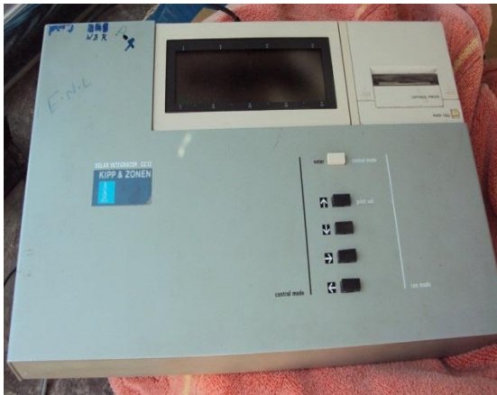
Fig.32 Digital display of Pyranometer
