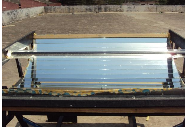
Fig.24 Reflector with absorber tube
