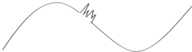
Figure-2.5: Oscillatory Transient
