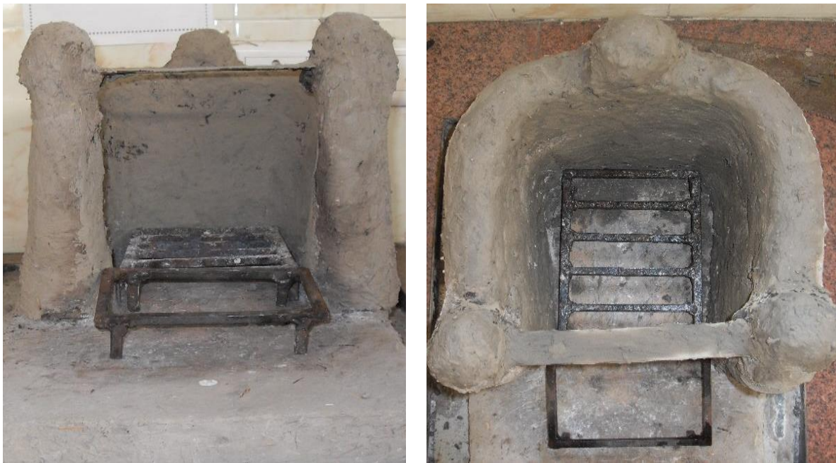
Fig. 4.1: Photographic views of the modified traditional cookstove (NIRE 02)
