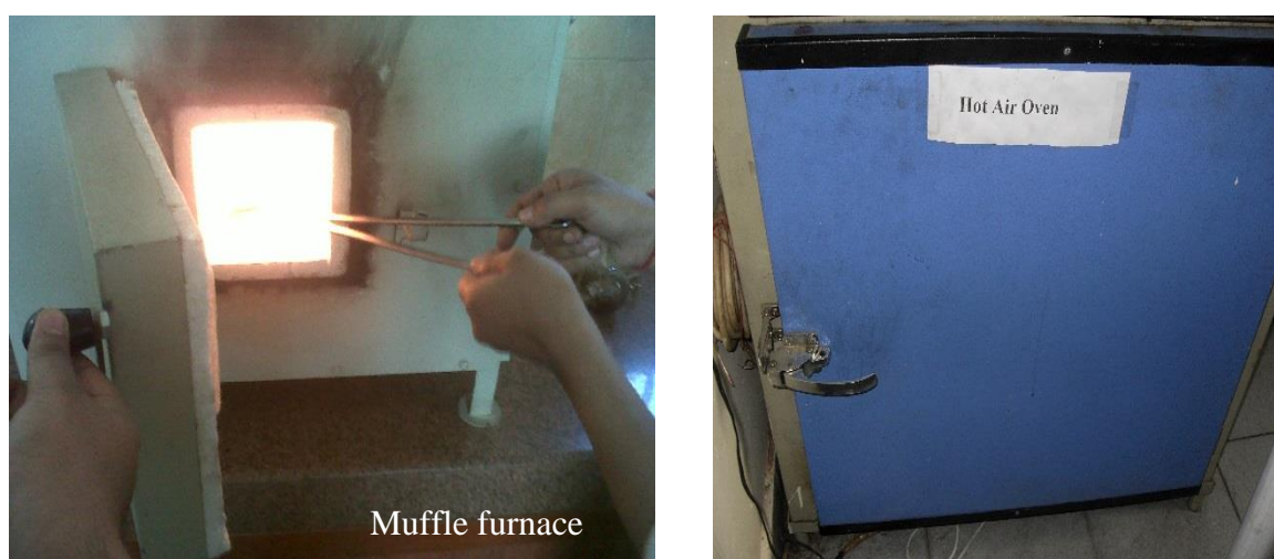
Fig. 4.8: Muffle furnace used for proximate analysis and Hot air oven for moisture reduction.
