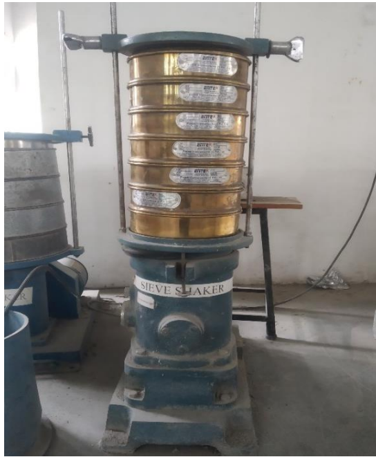
Figure 3. 3 Arrangement of sieves for sieve analysis of fine aggregates
