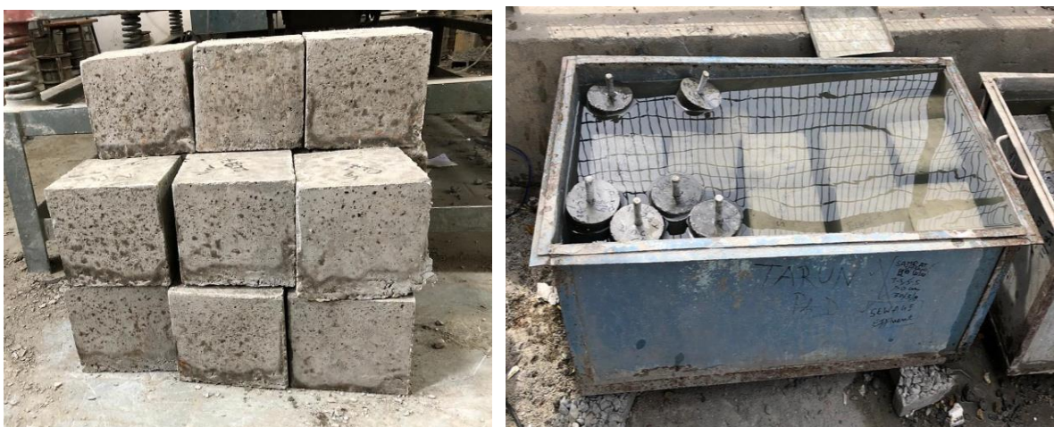
Figure 3. 7 Unmolded cubes and curing of the samples in respective medium.
