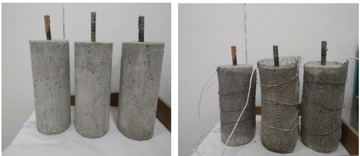
Figure 3. 16 Samples for corrosion testing
