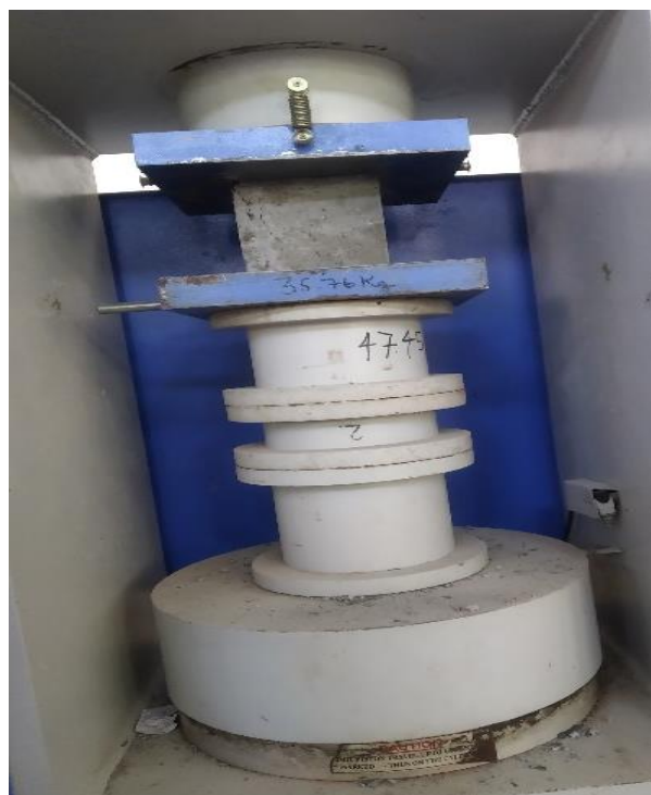
Figure 3.11 Compression testing machine for cube testing
