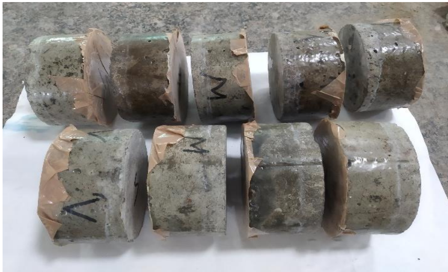
Figure 3. 14 Samples prepared for sorptivity test
