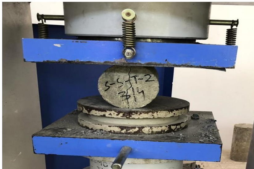
Figure 3.12 Split tensile strength test
