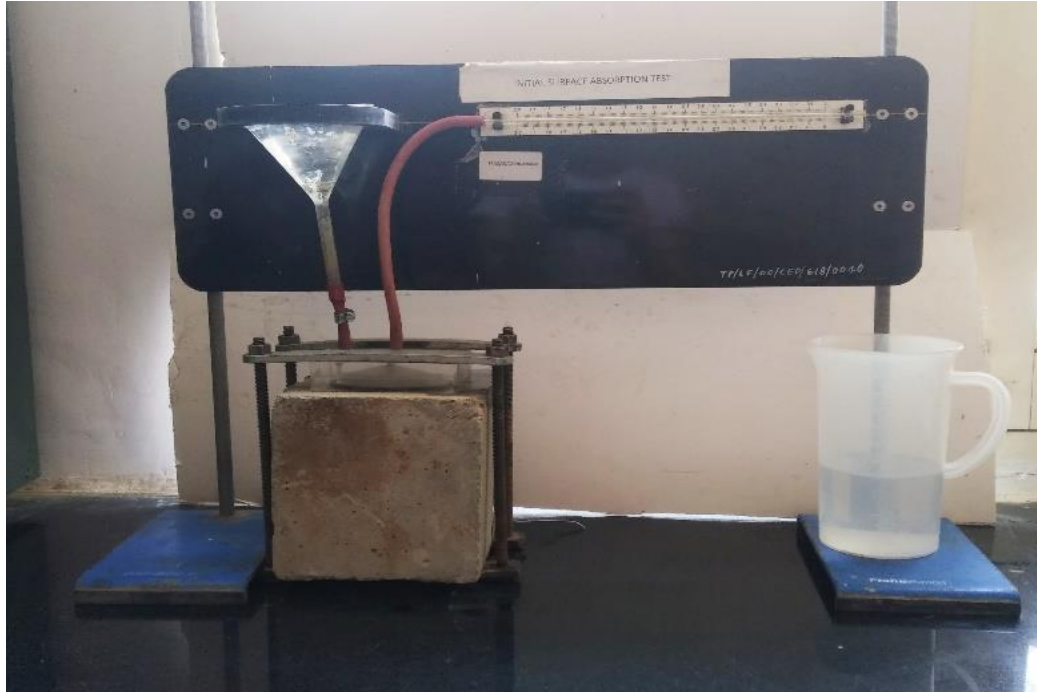
Figure 3. 13 Setup for ISAT test
