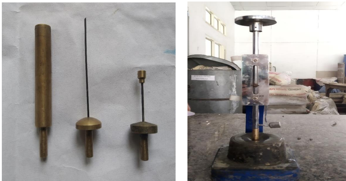
Figure 3.9 Different needle attachments of Vicat apparatus and Vicat apparatus fitted with consistency attachment
