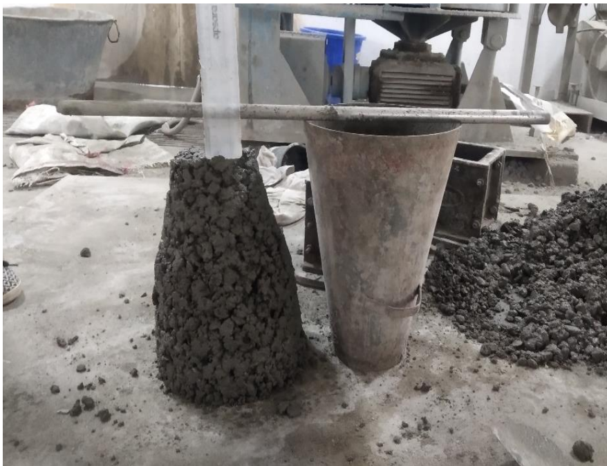
Figure 3. 10 Slump test apparatus
