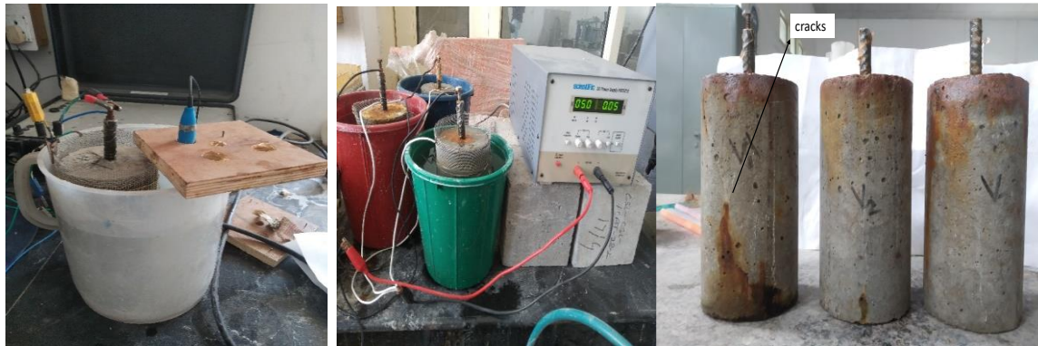
Figure 3.17 Setup for corrosion testing and corroded samples with cracks
