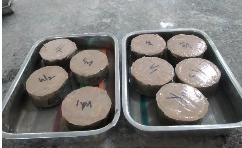
Figure 3. 15 Setup for sorptivity test
